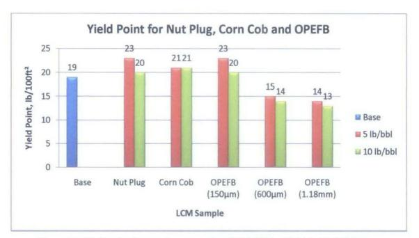
Figure 4.2 - Yield point for nut plug, corn cob and OPEFB in 5 lb/bbl and 10 lb/bbl
