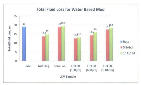
Figure 4.6 - Total fluid loss for water based mud
