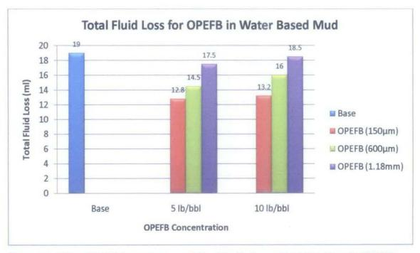
Figure 4.8 - Effect of LCM Concentration and Size Distribution on Total Fluid Loss for OPEFB in Water Based Mud
