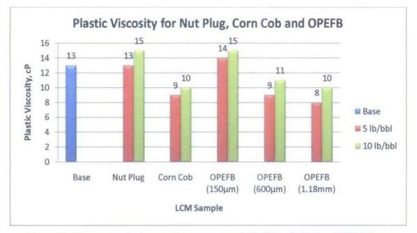
Figure 4.1 - Plastic viscosity for nut plug, corn cob and OPEFB in 5 lb/bbl and 10 lb/bbl
