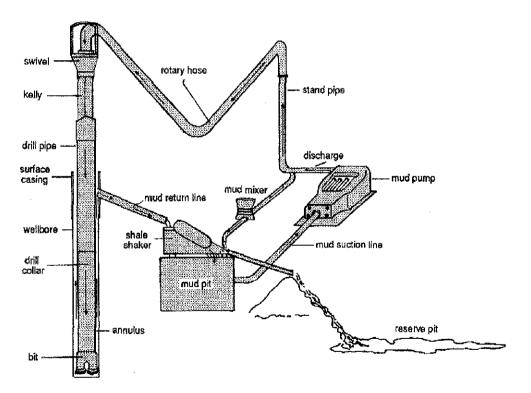
Figure 2.2 - Diagram illustrating the drilling –fluid (drilling mud) system and the flow of the fluids through the system
