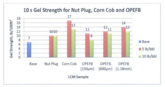
Figure 4.3 - 10-second gel strength for nut plug, corn cob and OPEFB in 5 lb/bbl and 10 lb/bbl
