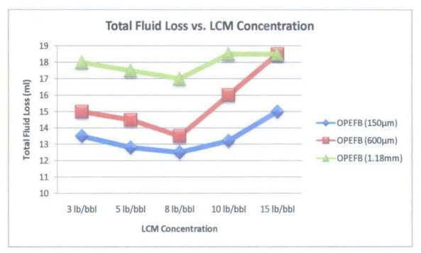
Figure 4.7 - Total Fluid Loss vs. LCM Concentration
