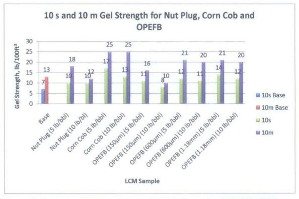
Figure 4.5 - 10-second and 10-minute gel strength for nut plug, corn cob and OPEFB in 5 lb/bbl and 10 lb/bbl
