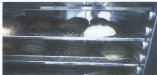
Figure 7- Coconut Shell Drying in Oven
