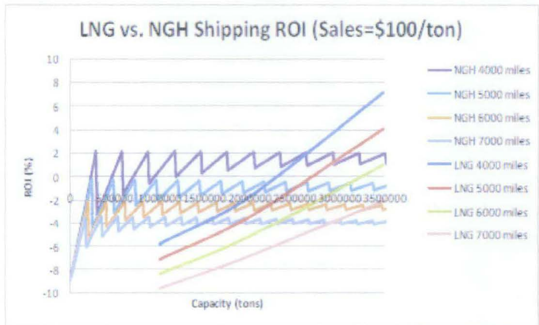
Fig A6 Graph of natural gas hydrate and liquefied natural gas shipping capacity vs. ROI
