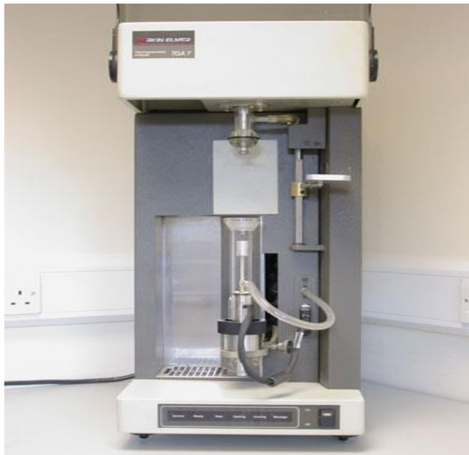
Figure 2.2: The example of thermal gravimetric analyzer. Source from http://www.materials.co.uk
