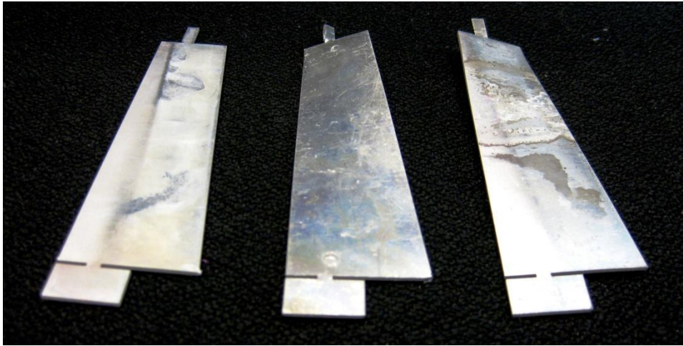
Figure 3-10: (From Left to Right) Straight Blade, Forward-Twist-Blade and Backward-Twist-Blade
