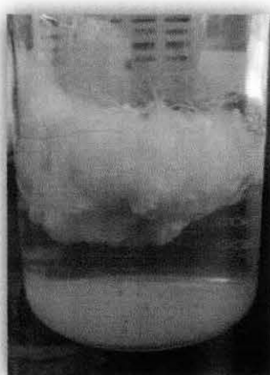
Figure 28 : Kapok – Diesel oil absorbency test
