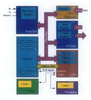
Figure 1: Microcontroller basic block diagram
