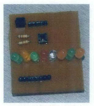
Figure 17: LEDs add-on board
