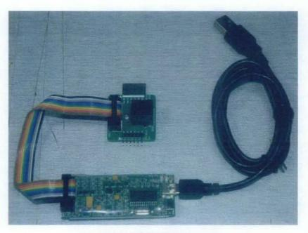
Figure 12: PIC USB Programmer
