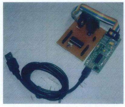
Figure 13: Connected main board with programmer
