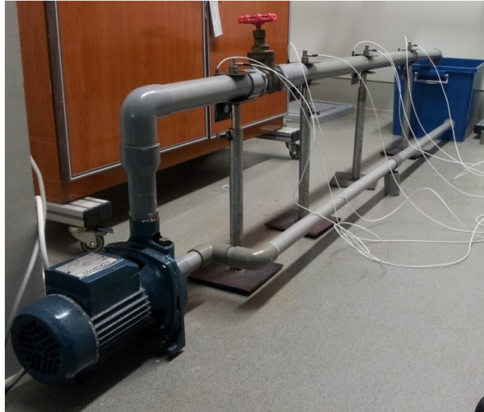
Figure 3.3: Experiment equipped with accelerometer on the pipe support for testing section of 4.540 cm diameter pipe
