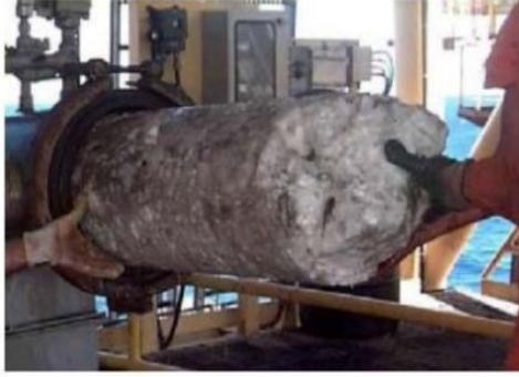
Figure 1.2: Hydrate formation in natural gas transmission pipeline [2]
