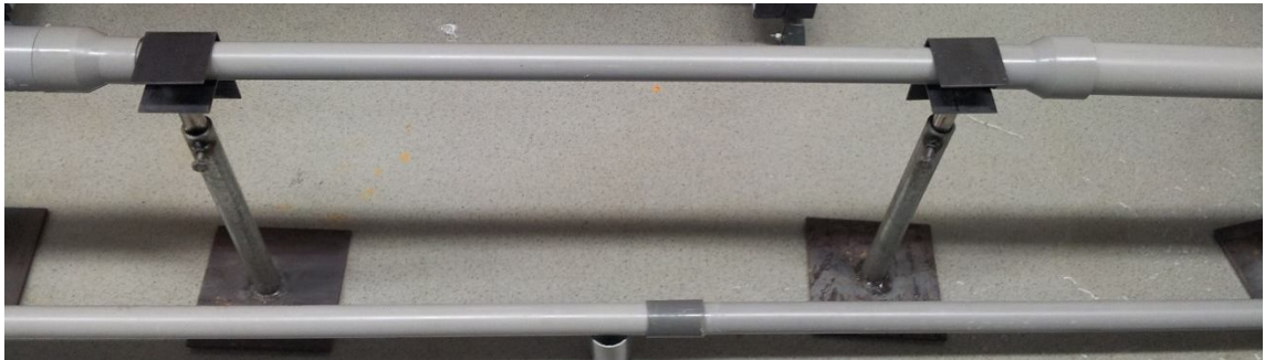
Figure 3.4: Testing Section using 3.004 cm diameter pipe
