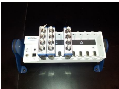
Figure 3.9: Data Acquisition, cDAQ-9172 and Analog Input Modules 9215
