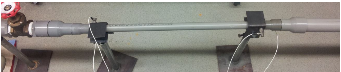
Figure 3.5: Testing Section using 2.494 cm diameter pipe
