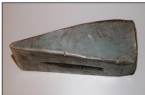
FIGURE 4: The wedge placed under the fixture to incline the plane [11]
