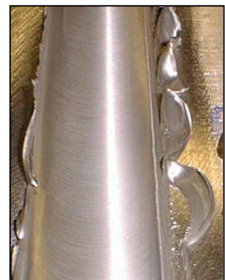
FIGURE 7 : Flash ribbon deposited outside the weld joint [14]
