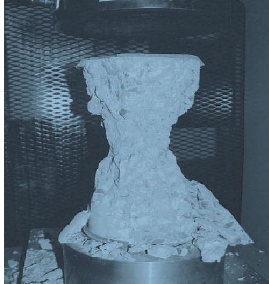
Figure 1: Fractured Test Specimen at Failure
