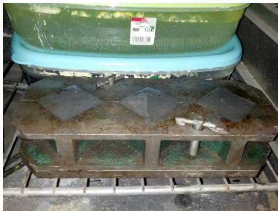
Figure 7: Molded slurry is put into oven for curing process
