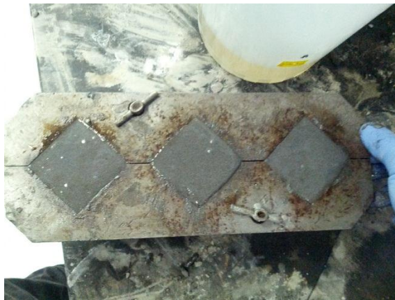
Figure 6: Slurry is put into 50mm x 50mm mold
