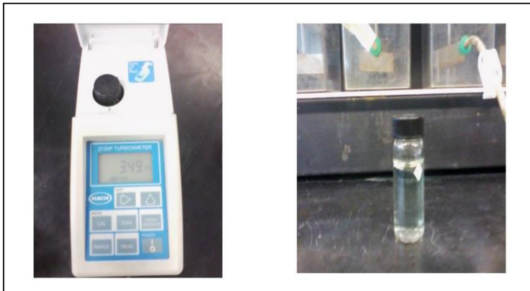
Figure 19 : Mixture Solution and Turbidimeter
