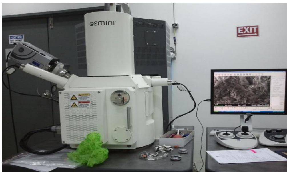
Figure 9: Supra 55VP Zeiss Variable Pressure Field Emission Scanning Electron Microscope (VP-FESEM)
