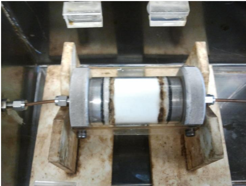
Figure 13: Unconsolidated cores column setup for characterization and coreflooding experiment
