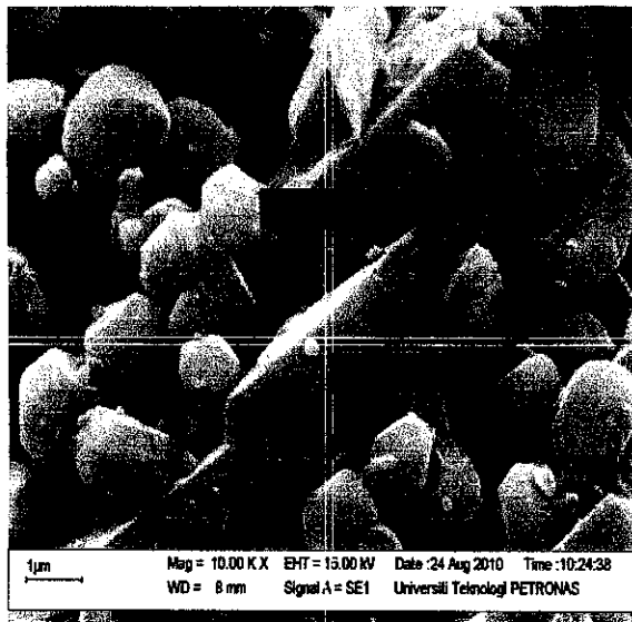
Figure 16: SEM Photograph for Fe-Co/Al 2 O 3 (sequential)
