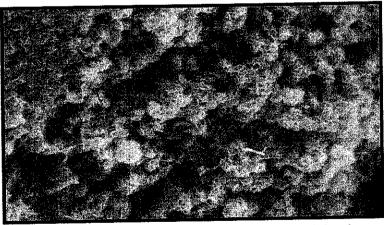
Figure 30: SEM 10000X catalyst 4.0 after calcined.
