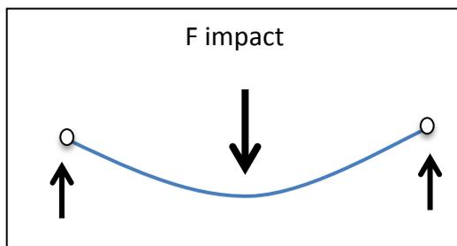
**Figure 23: Top view of landing net during impact**
