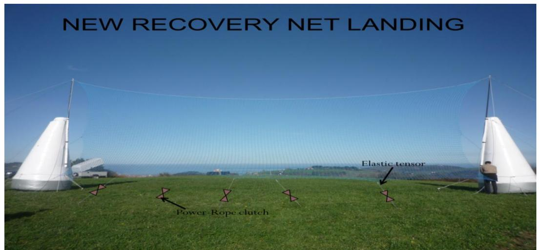
**Figure 37: Design Concept New Recovery Net landing**
