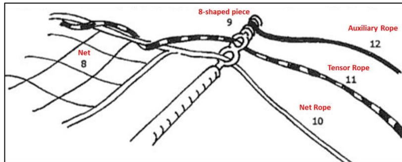
**Figure 17: Auxiliary, Tensor rope and Net**
