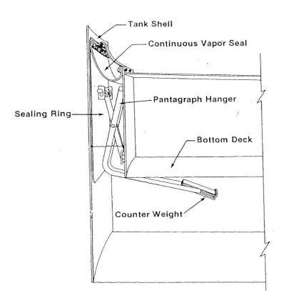
Figure 4: Roof Seal Component.
