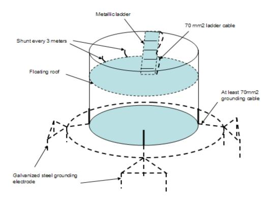
Figure 5: Overview of FRT Grounding system.
