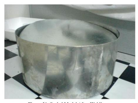
Figure 21: Scaled Model After Welding.
