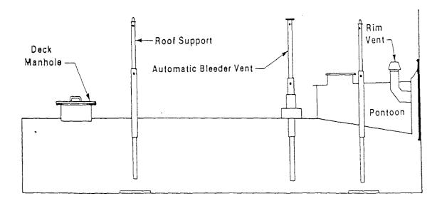
Figure 3: Tank Roof Fittings.
