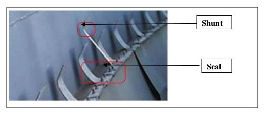
Figure 1: Locations of Shunt and Seal.
