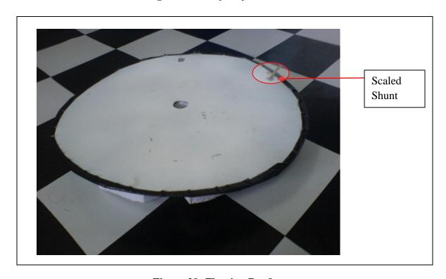
Figure 29: Floating Roof.
