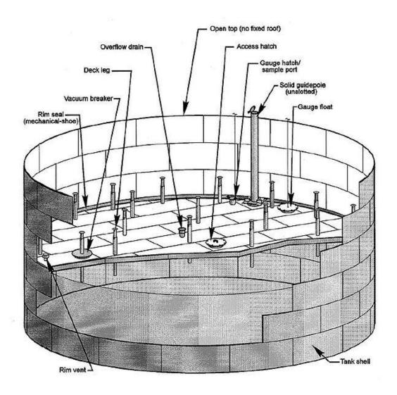
**Figure 2: Floating Roof Tank Components.**
