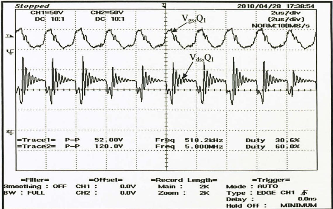
Figure 29  $V_{gs, Q_1}$  and  $V_{ds, Q_1}$  for switching frequency of 510.2kHz
