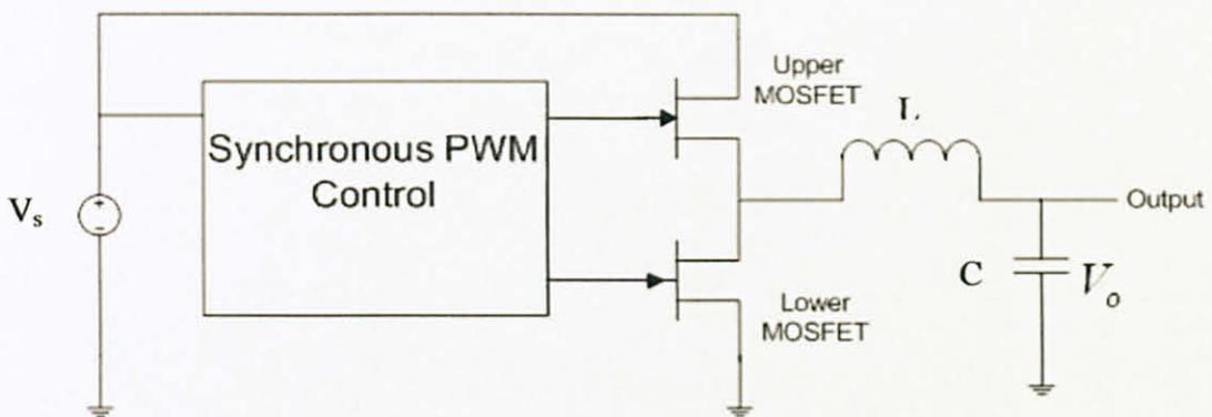
Figure 4 Synchronous buck-converter topology [10].
