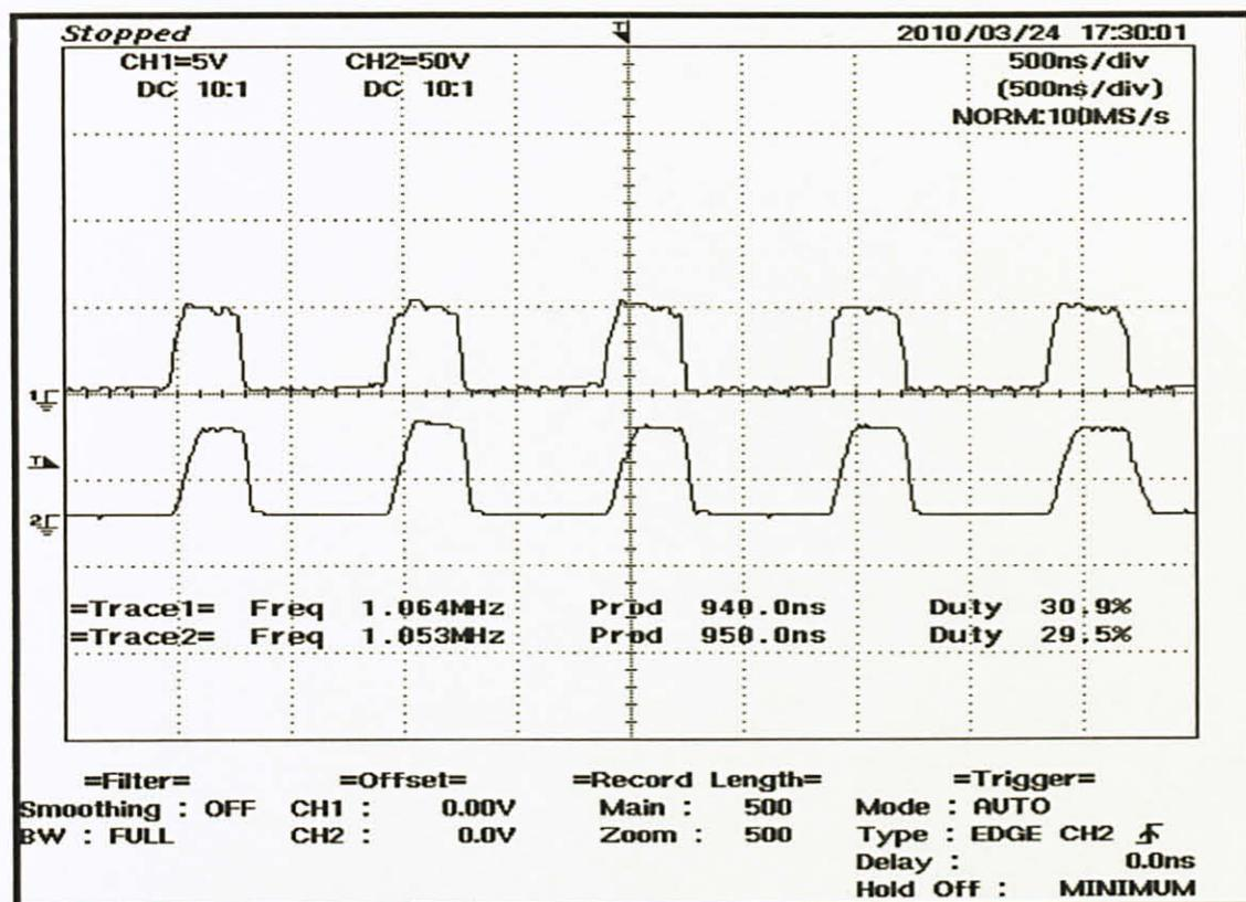
Figure 24 Synchronized PWM output waveform [X: 500ns/div, Y: 5V/div]
