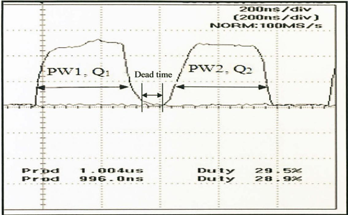
Figure 26 Synchronized signals of  $PW_1$  and  $PW_2$ , duty ratio of 30%
