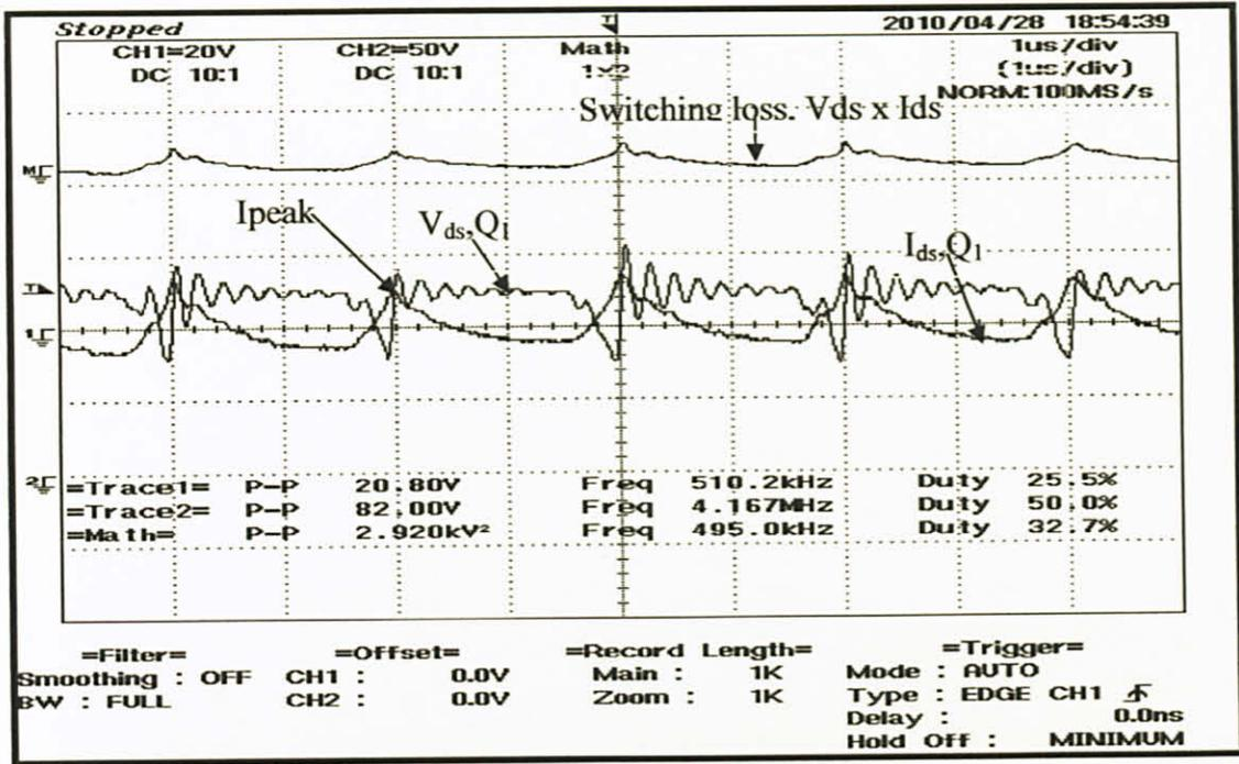
Figure 30  $V_{ds}$ ,  $I_{ds}$  and switching loss for  $Q_1$
