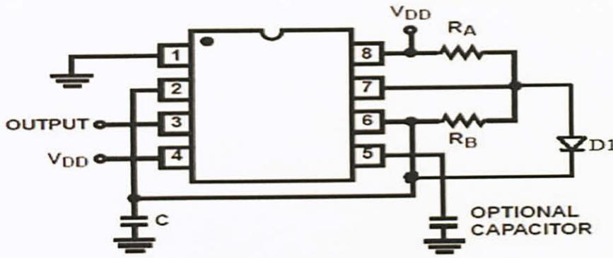
Figure 12 Modified astable circuit chip [7]
