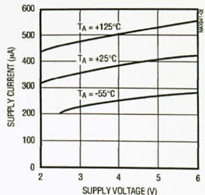
**MAX942 TOTAL SUPPLY CURRENT vs. SUPPLY VOLTAGE**
