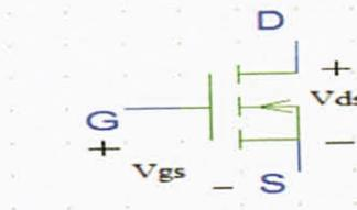
Figure 6 Symbol for N-channel MOSFET [6]
