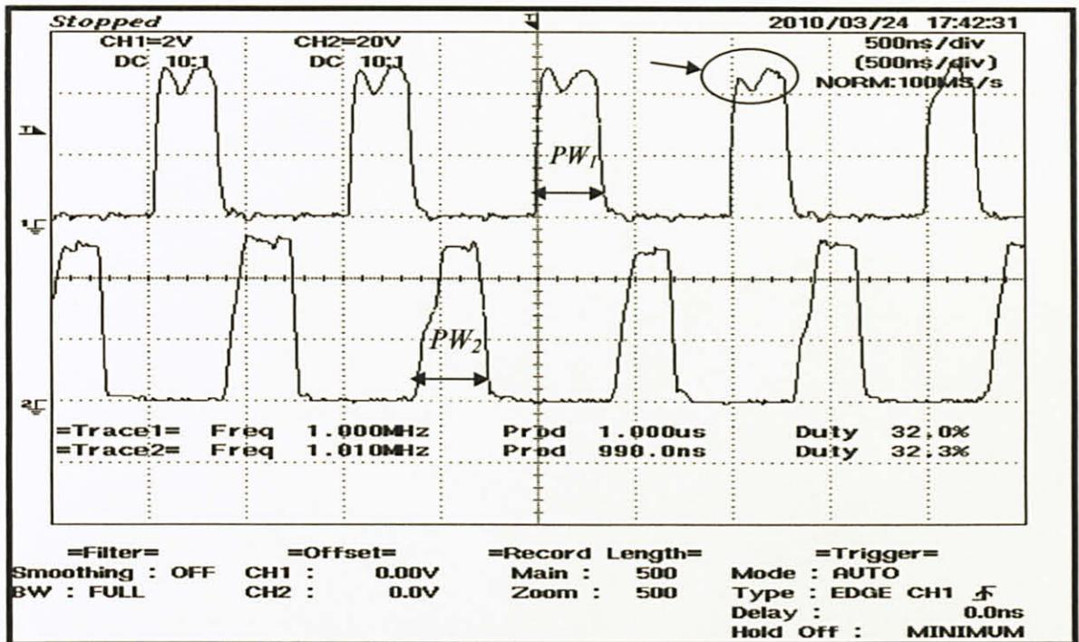
Figure 25 Two synchronized signal after delay line circuit being applied [X: 500ns/div, Y: 2V/div]
