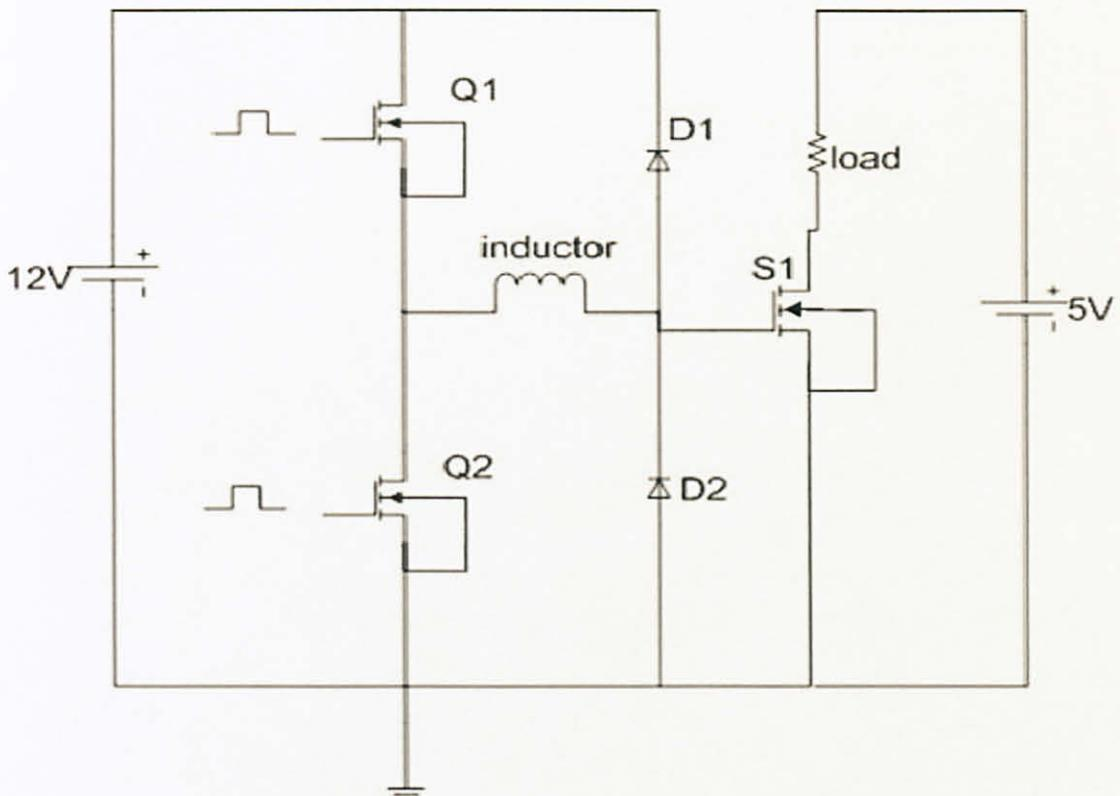
Figure 18 Schematic for DC-RGD circuit
