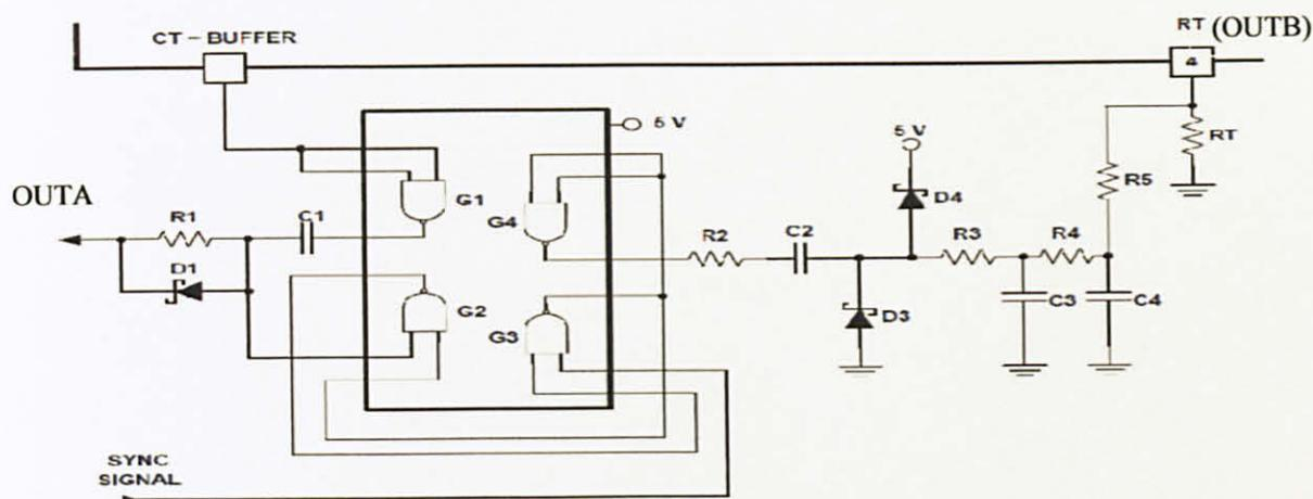
Figure 15 The configuration for synchronization circuit [11]
