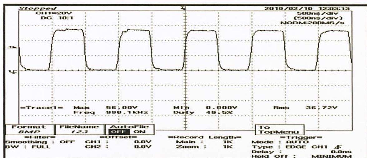
Figure 22 The experiment result showing 49.5% duty ratio [X: 500ns/div, Y: 2V/div]
