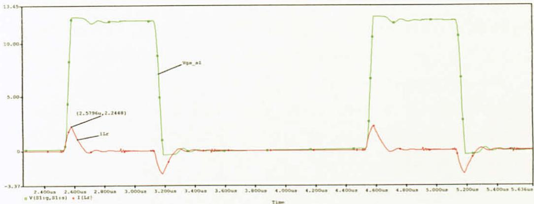
Figure 35 Graph of  $V_{gs\_S1}$  and resonant inductor current,  $i_{Lr}$
