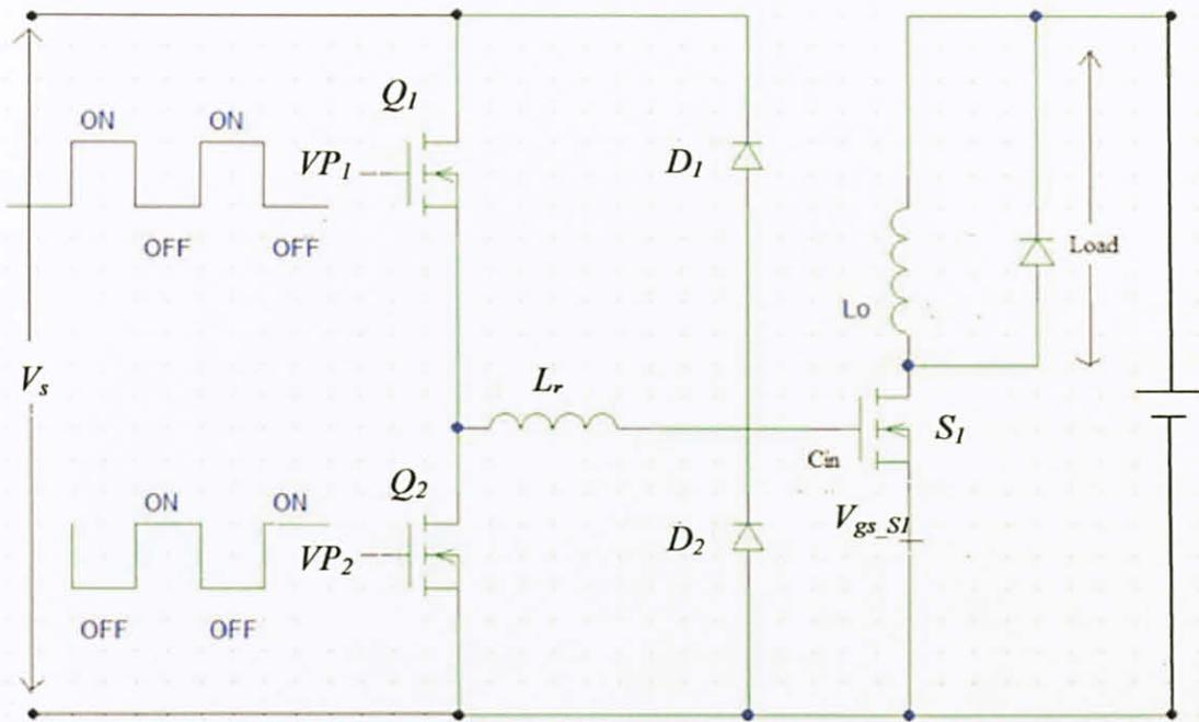
Figure 5 The diode-clamped resonant gate driver with voltage pulses[2]
