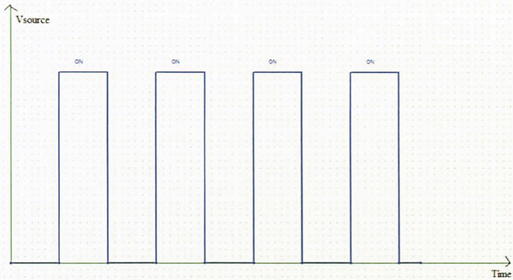
Figure 1 The example of PWM signal
