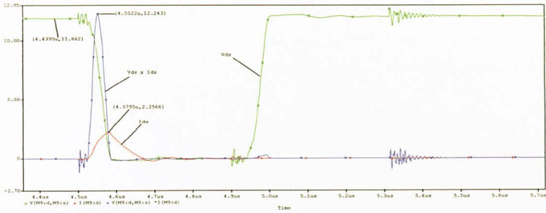
Figure 34 Simulation of  $V_{ds}$  and  $I_{ds}$  for  $Q_1$  and switching loss
