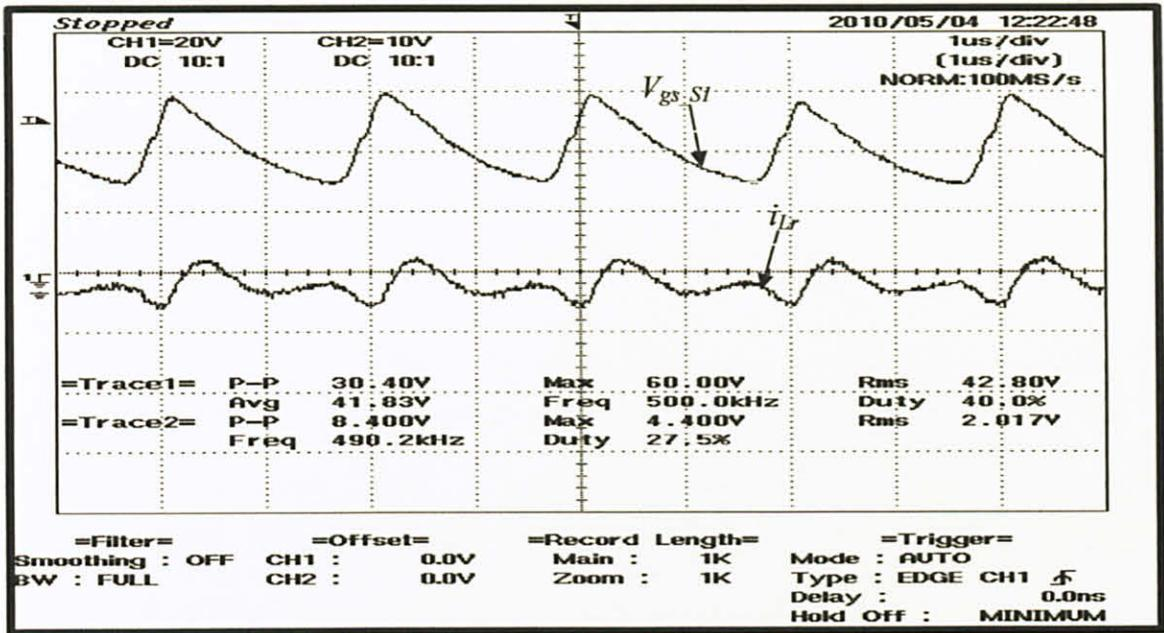
Figure 31 Graph of  $i_{Lr}$  of 10nH and  $V_{gs\_S1}$ , within 400ns pulse width
