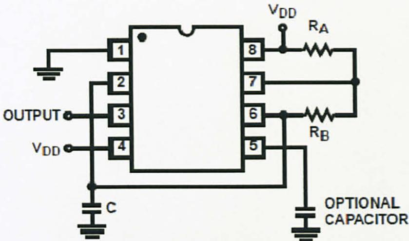
Figure 11 Astable circuit chip [7]
