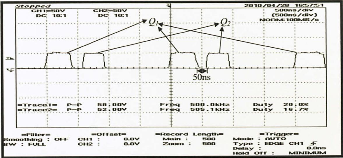
Figure 27  $V_g$  applied respectively to both switches  $Q_1$  and  $Q_2$  [X:500ns/div, Y:5V/div]
