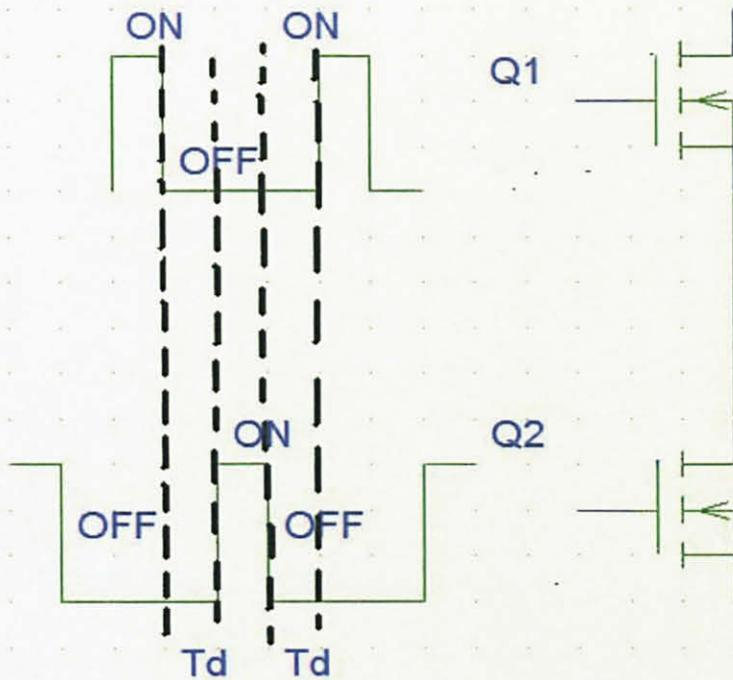
Figure 2 Synchronous switching using PWM
