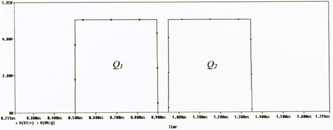
Figure 32 Pulse width of  $Q_1$  and  $Q_2$  within 400ns each (20% duty ratio)
