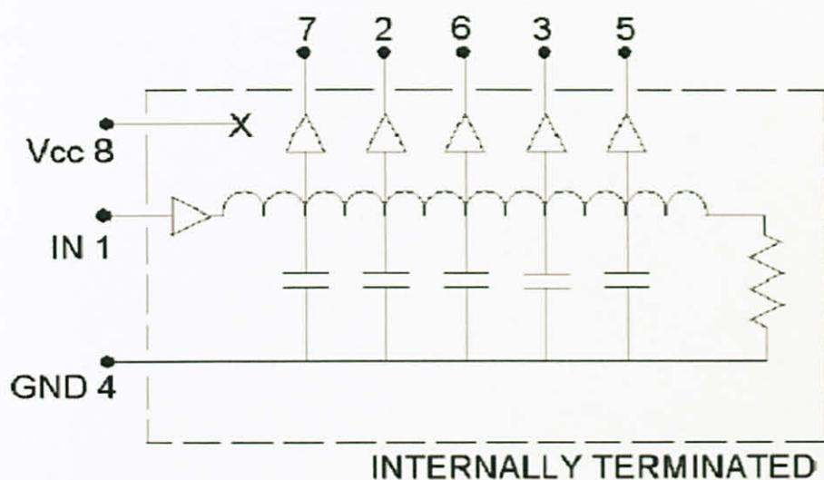
Figure 16 Layout for the delay line (see appendix D for details)
