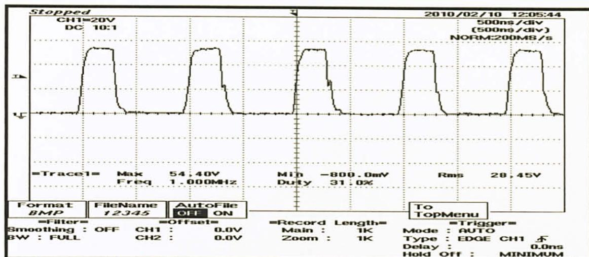
Figure 20 The experiment result showing 31.0% duty ratio [X: 500ns/div, Y: 5V/div]
