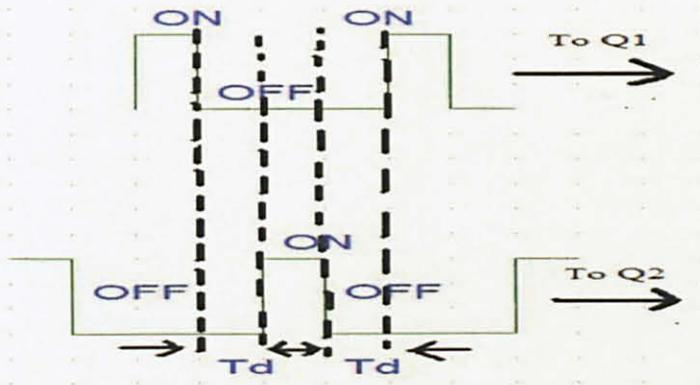
Figure 3 The effect of dead time on driving pulses
