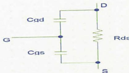
Figure 7 MOSFET equivalent circuit in the ohmic region [6]
