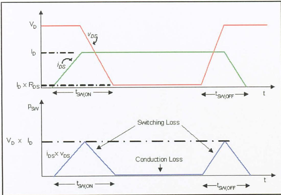
Figure 8 Switching losses occurs as MOSFET's transition between fully ON and fully OFF [8]
