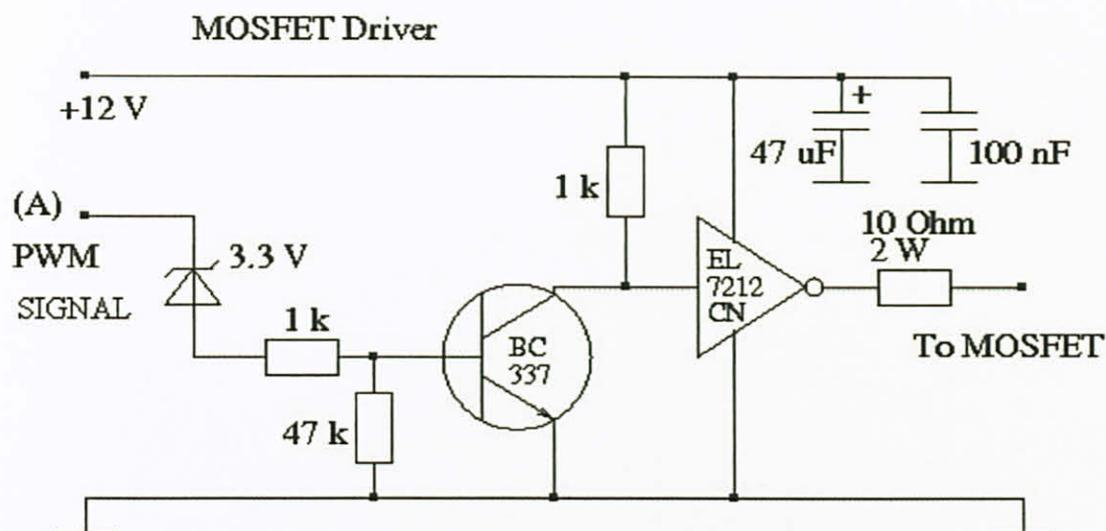
Figure 17 Circuit layout for MOSFET driver [12]
