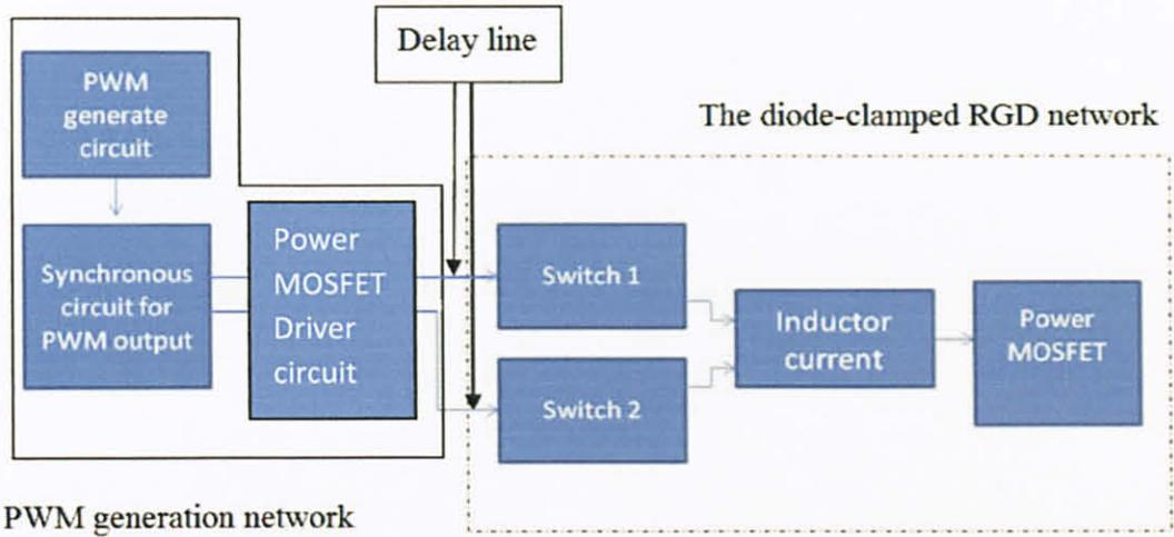
Figure 10 Proposed block diagram for overall circuit
