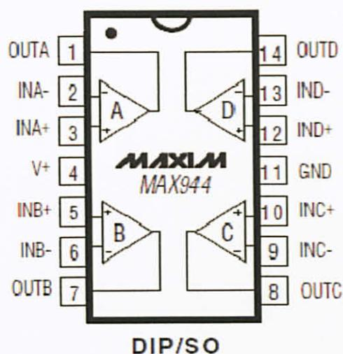
Figure 14 MAX944 pin layout (see appendix C for details)
