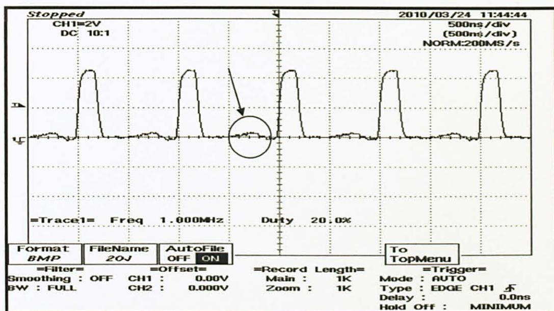
Figure 19 The experiment result showing 20.0% duty ratio [X: 500ns/div, Y: 2V/div]
