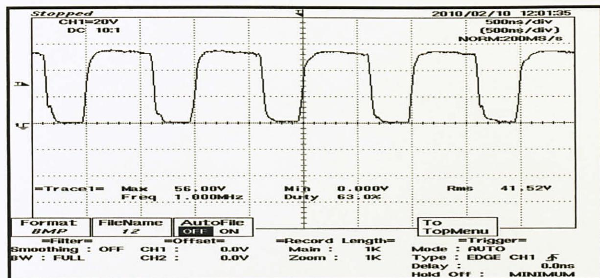
Figure 23 The experiment result showing 63.0% duty ratio [X: 500ns/div, Y: 2V/div]
