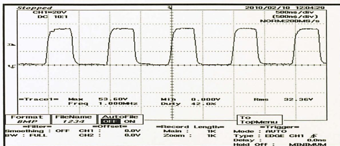
Figure 21 The experiment result showing 42.0% duty ratio [X: 500ns/div, Y: 2V/div]
