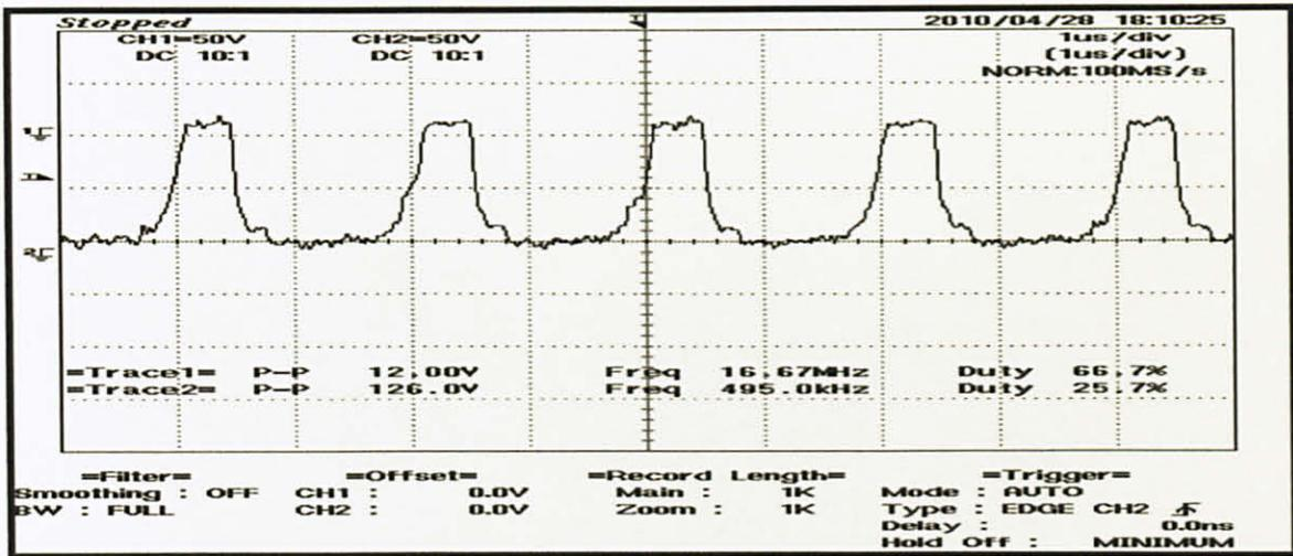
Figure 28 Pulse width 1 ( $VP_1$ ) applied to the driving gate of switch  $Q_1$  [X:1us/div, Y: 5V/div]
