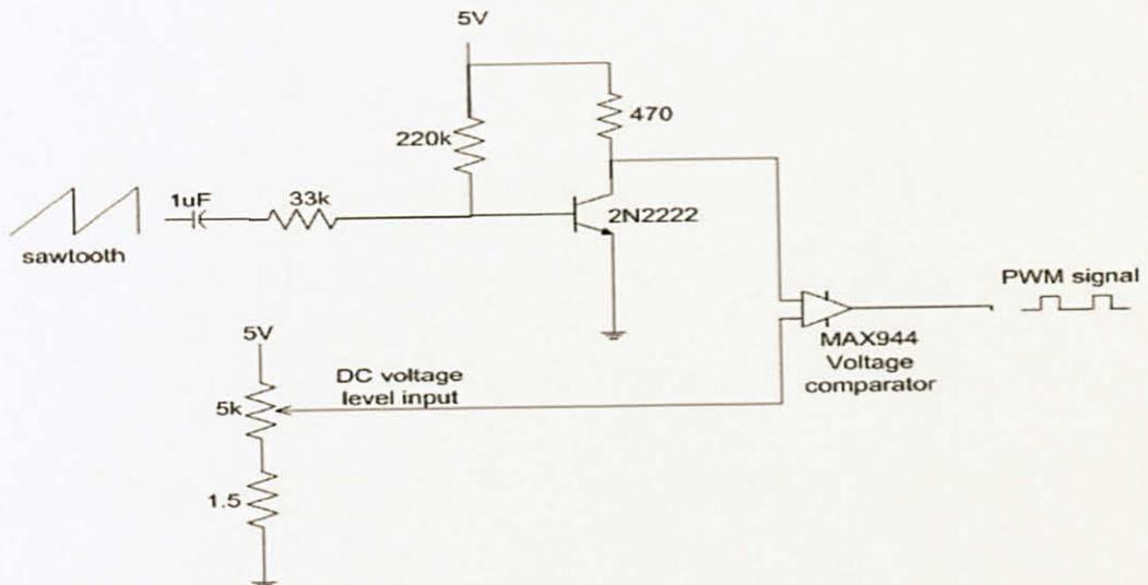
Figure 13 Voltage controlled PWM generator schematic [11]
