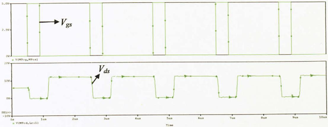
Figure 33  $V_{gs}$  and  $V_{ds}$  of switch  $Q_1$  in DC-RGD circuit
