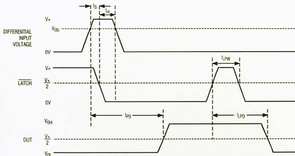
Figure 2. MAX941 Timing Diagram with Latch Operator
