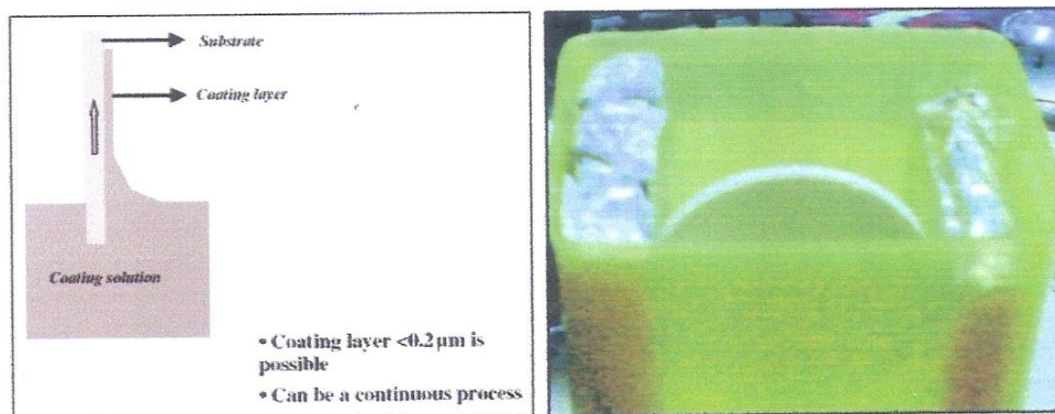
Figure 3.2 : Dip-coating method of the porous alumina support in silica sol
