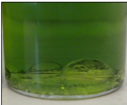
Figure 4: The formation of droplets settle at the bottom of methanol rich phase at 50% conversion
