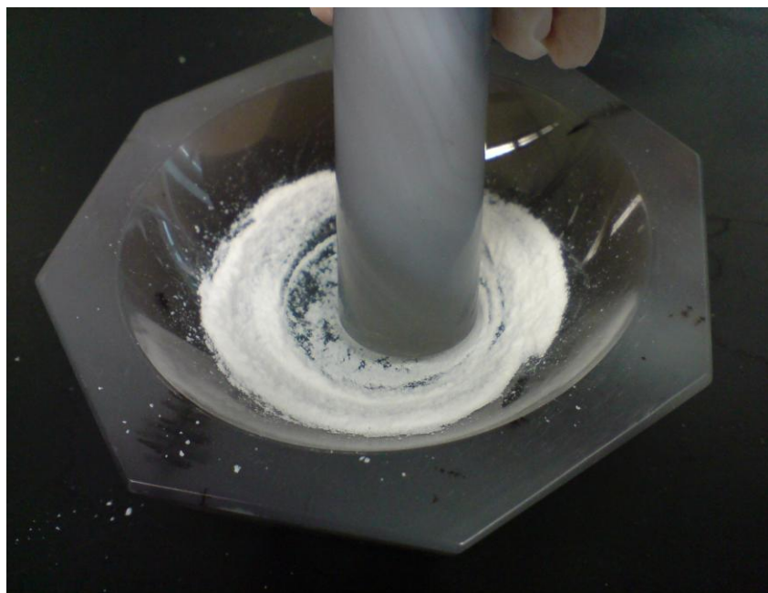
Figure C7: Grinding Process to Form fine Nano silica
