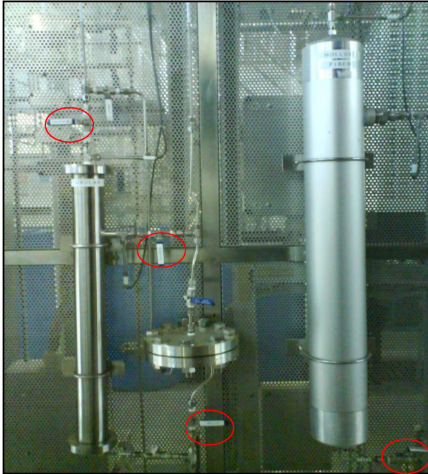
Figure 3. 1: Tubular and Hollow-Fiber Module
