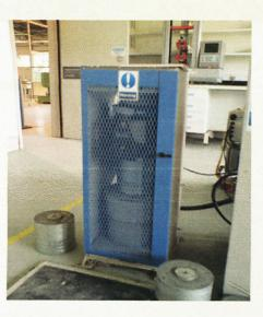
Figure 4.1.3: 2000 kN Compression and Flexural Machine
