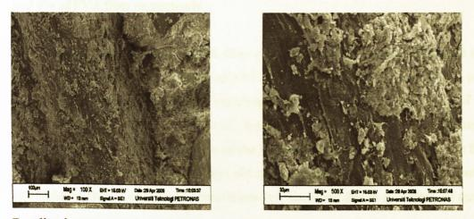
Bonding between PVA fiber and cement after 435 days → 100 X and 500 X zoom
