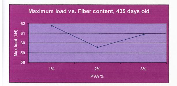
Figure 4.2.1: Maximum load versus fiber content
