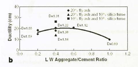
Figure 2.3.2: Effect of lightweight aggregate content on ductility
