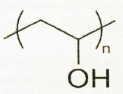
Figure 2.1: Chemical structure of polyvinyl alcohol (PVA)
