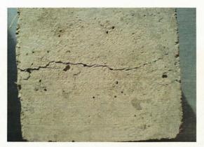
Figure 4.1.2: Line of failure of sample
