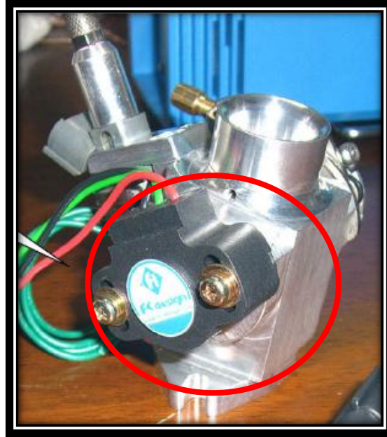
Figure 19: Throttle Position Sensor (TPS) [9]
