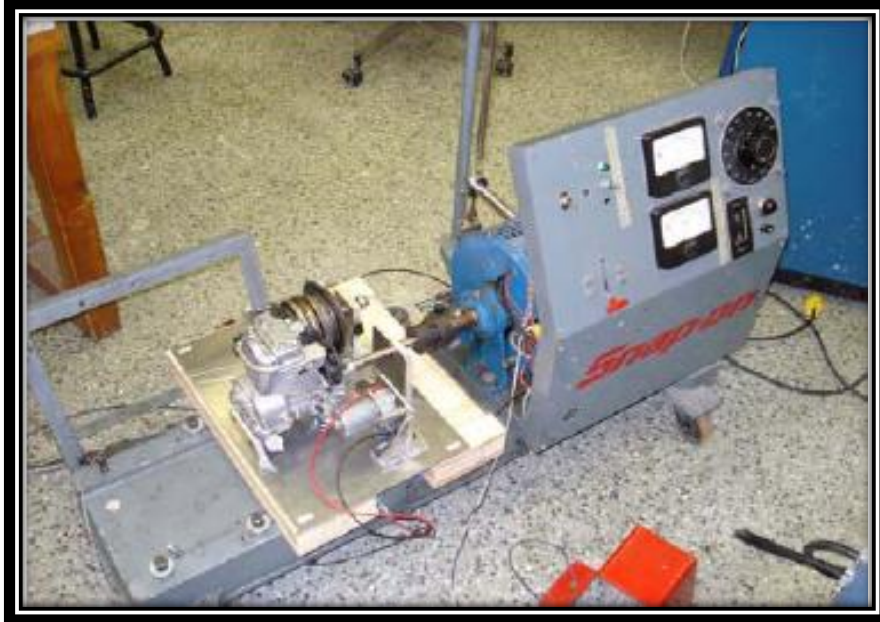
Figure 6: Dynamometer and engine assembly [10]
