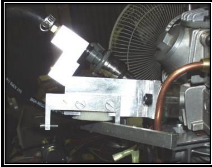
Figure 11: Throttle body with injector [7]
