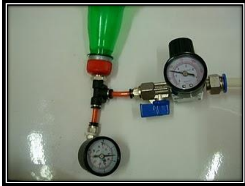
Figure 15: Pressure gauge attach to temporary fuel tank
