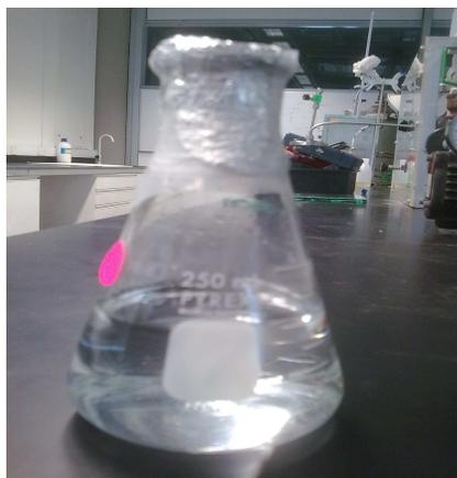
Figure 3.5: Tetraorthosilicate (TEOS) solution prepared.
