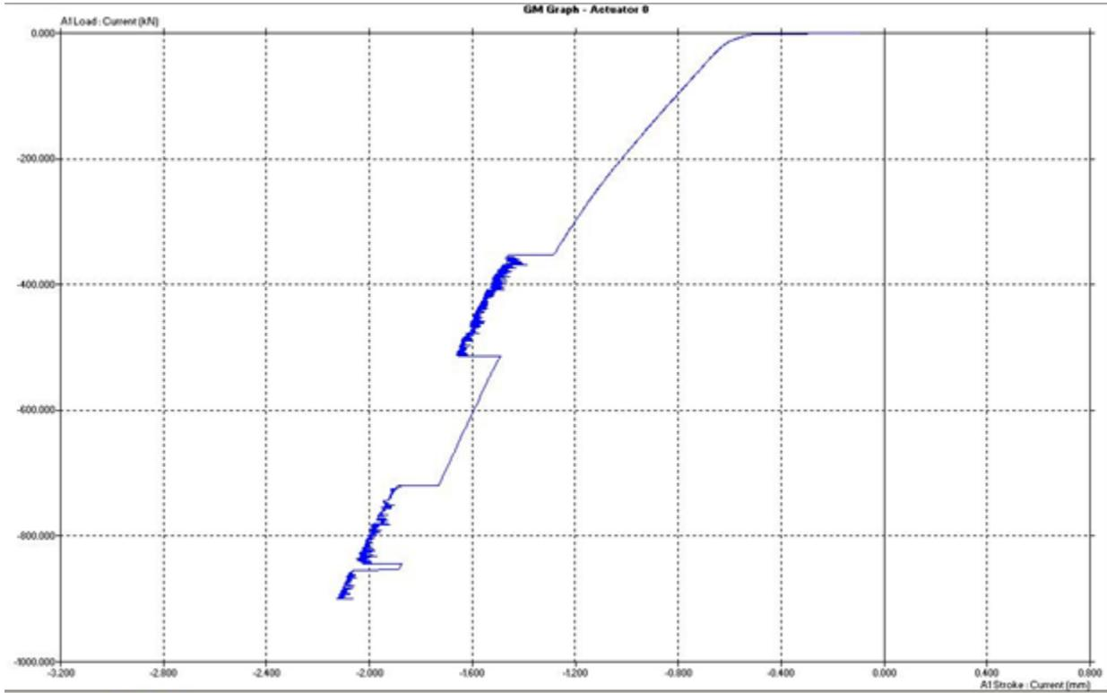
Appendix 4. load vs. deflection for 3.43% corroded specimen
