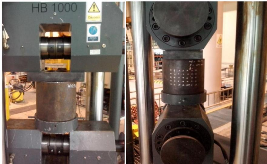
**Figure 6 UTM testing of the pipeline (left no pitting, right with pitting corrosion)**
