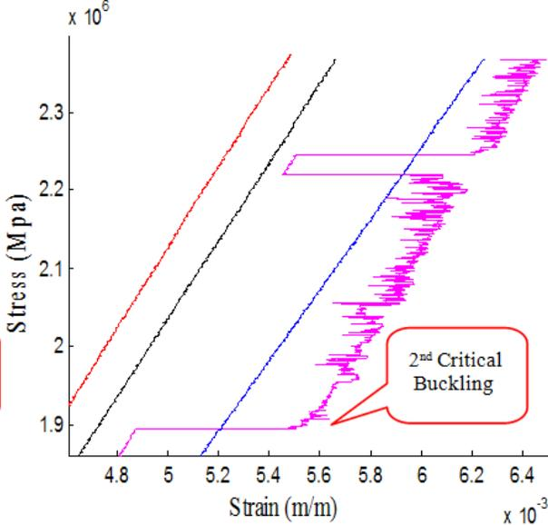
Figure 17 Second Critical Buckling
