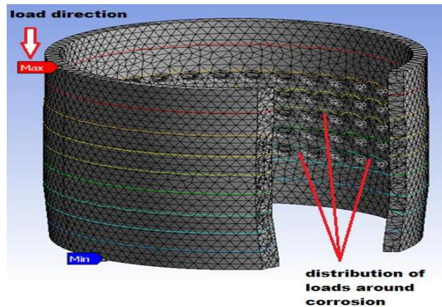
**Figure 26 Load distribution around corrosion**
