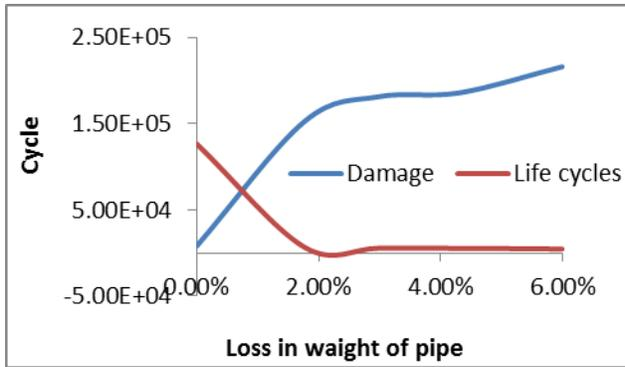
Figure 24 Damage/Life vs. corrosion ratio
