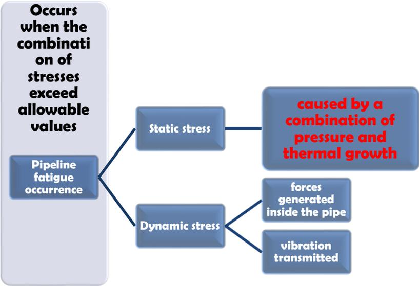
Figure 4 Pipeline fatigue occurrence
