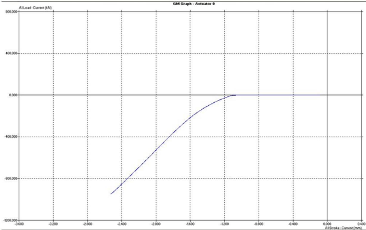
Appendix 2. load vs. deflection for 1.14% corroded specimen
