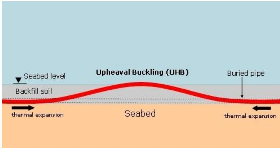
**Figure 1 Upheaval buckling**
