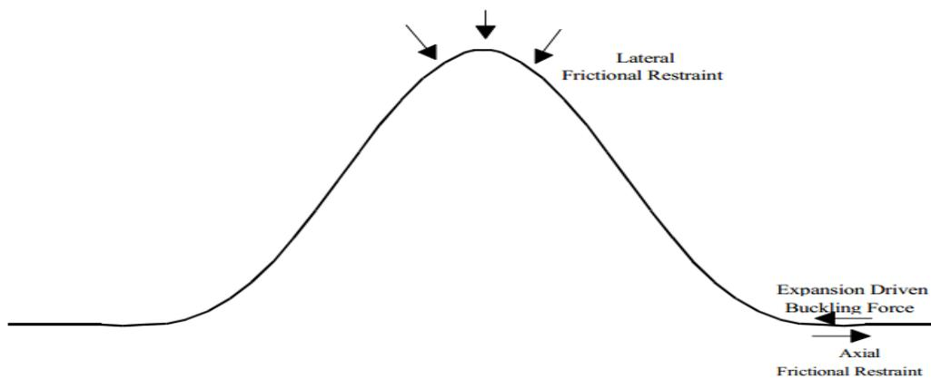
Figure 5 forces acting during upheaval buckling
