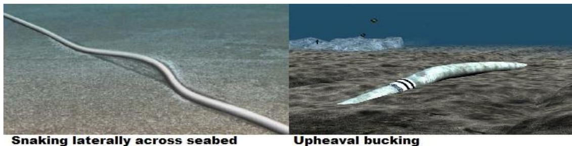
**Figure 2 types of buckling in seabedded pipelines**
