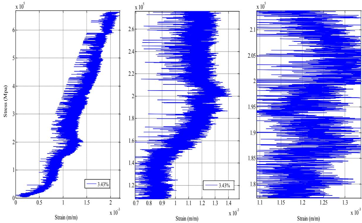
**Figure 20 Stress vs. Strain (3.43% corrosion ratio)**
