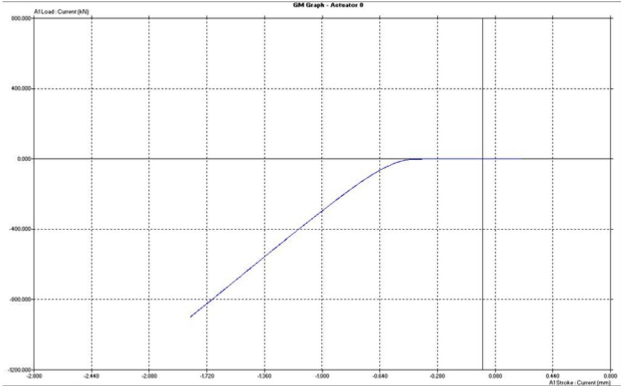
Appendix 3. load vs. deflection for 2.29% corroded specimen
