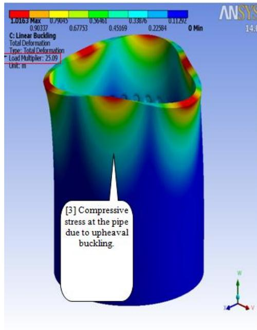
**Figure 21 Effect of 4.31% Corrosion Ratio**
