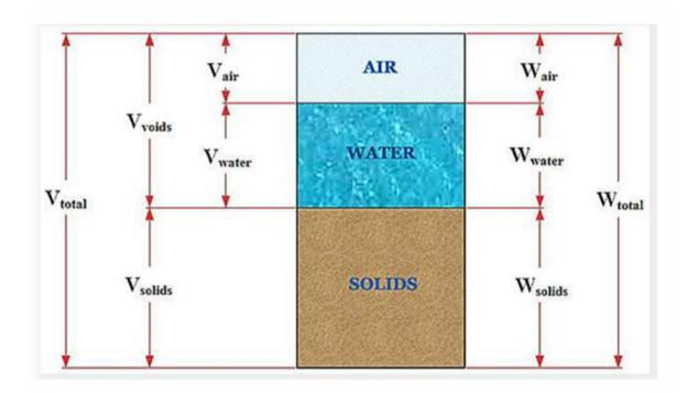
Figure 2.3.3: Phase Diagram of soil
