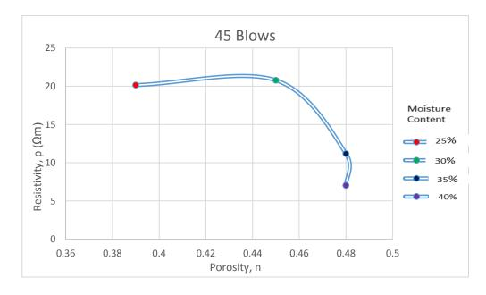
Figure 4.6: Resistivity vs Porosity for 45 Blows
