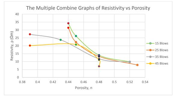
Figure 4.7: The Multiple Combine Graphs of Resistivity vs Porosity
