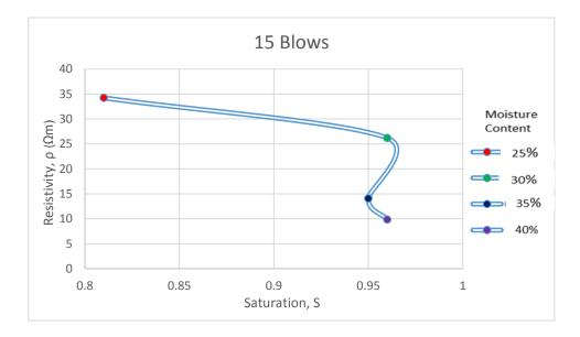
Figure 4.9: Resistivity vs Saturation for 15 Blows
