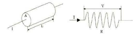
Figure 2.1: The schematics of cylindrical section and flow of current
