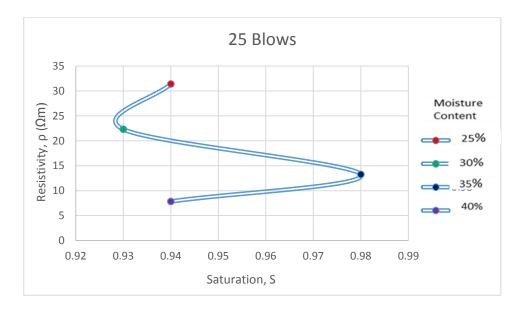
Figure 4.10: Resistivity vs Saturation for 25 Blows
