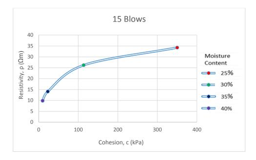
Figure 4.14: Resistivity vs Cohesion for 15 Blows
