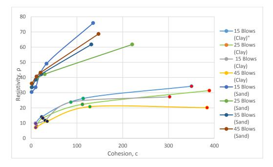
Figure 4.19: The Multiple Combine Graphs of Resistivity vs Cohesion (Clay and Sand)
