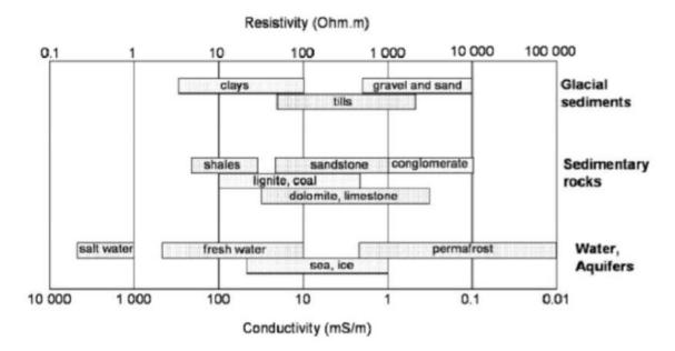
Figure 2.3.2: Typical range of electrical resistivity value of soil
