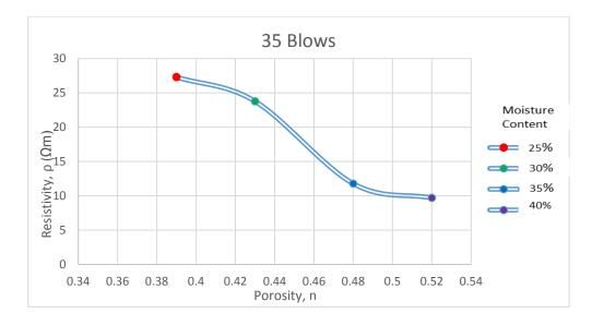
Figure 4.5: Resistivity vs Porosity for 35 Blows
