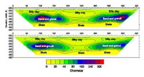
Figure 1.1: The Example of Mapping Stratigraphy, Sand and Gravel Lenses in Clay and Shale Environment
