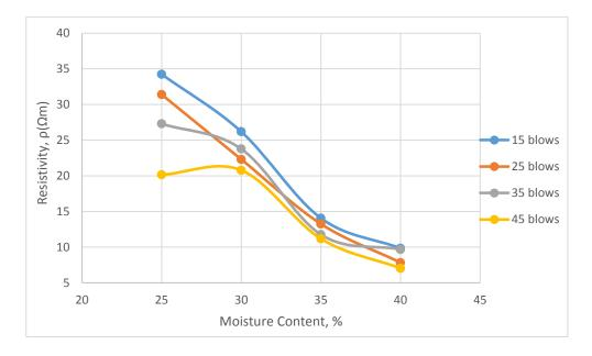
Figure 4.1: Resistivity vs Moisture Content
