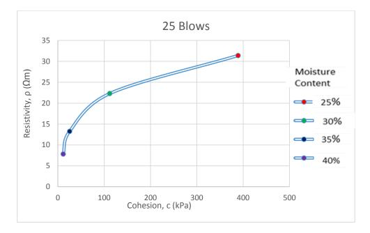
Figure 4.15: Resistivity vs Cohesion for 25 Blows
