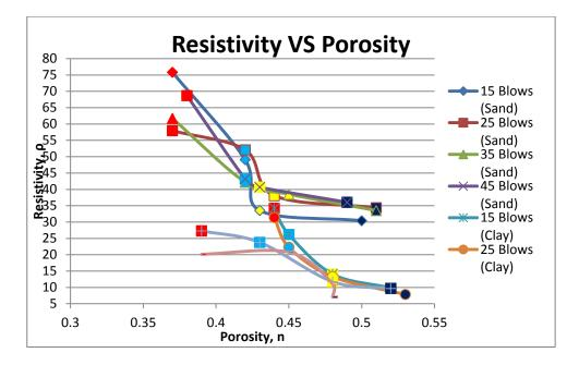
Figure 4.8: The Multiple Combine Graphs of Resistivity vs Porosity (Clay and Sand)
