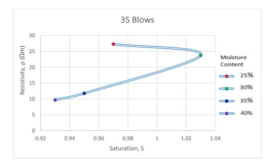
Figure 4.11: Resistivity vs Saturation for 35 Blows
