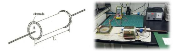
Figure 2.5.2: Laboratory Set Up for Soil Resistivity
