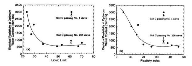
Figure 2.4.1: Relationship between Electrical Resistivity and Atterberg Limit at Optimum Water Content (Abu Hassanein et al., 1996)
