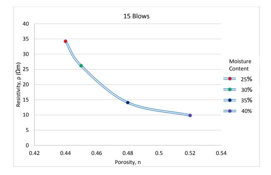
Figure 4.3: Resistivity vs Porosity for 15 Blows
