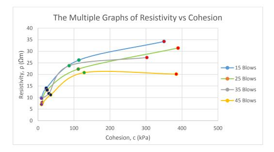
Figure 4.18: The Multiple Combine Graphs of Resistivity vs Cohesion
