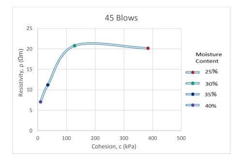
Figure 4.17: Resistivity vs Cohesion for 45 Blows
