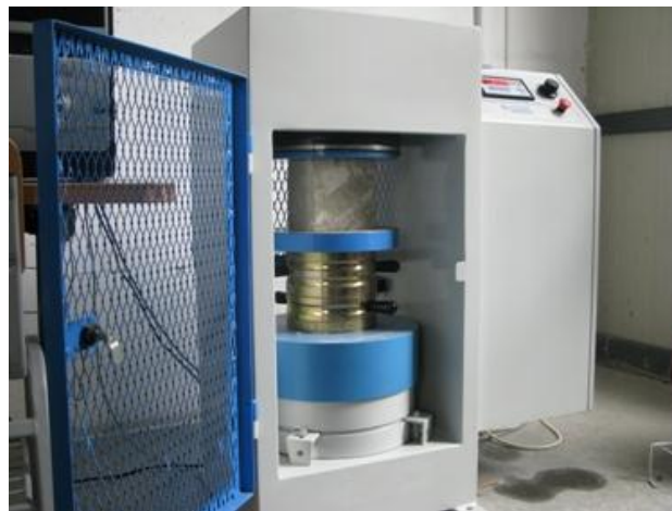
Figure 4.0 Compressive Strength Machine.
