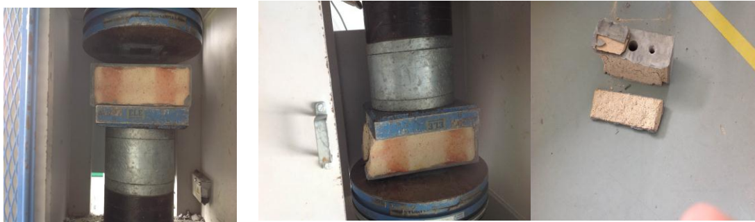
Figure 3.9 Shows the compressive strength test conducted on brick samples
