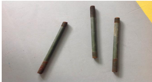
Figure 3.3 Steel rod for fastening inner brick layers.
