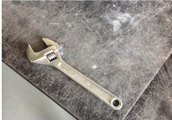
Figure 3.7 Crescent Wrench used for tightening the bolts.
