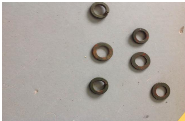
Figure 3.2 Washers to support the tightening of the bolts.
