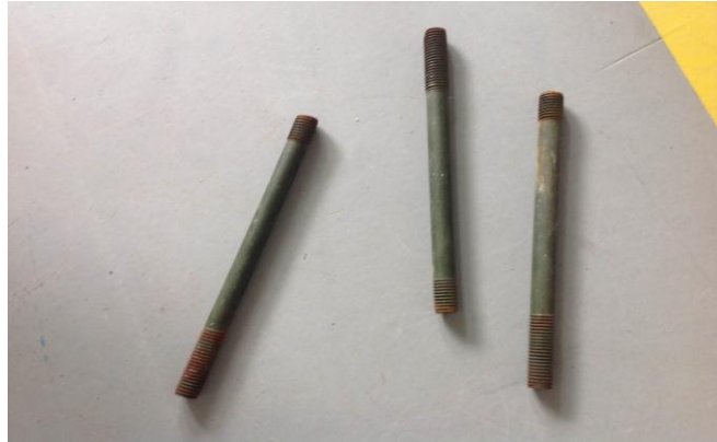
Figure 3.3 steel rods for fastening inner brick layers.
