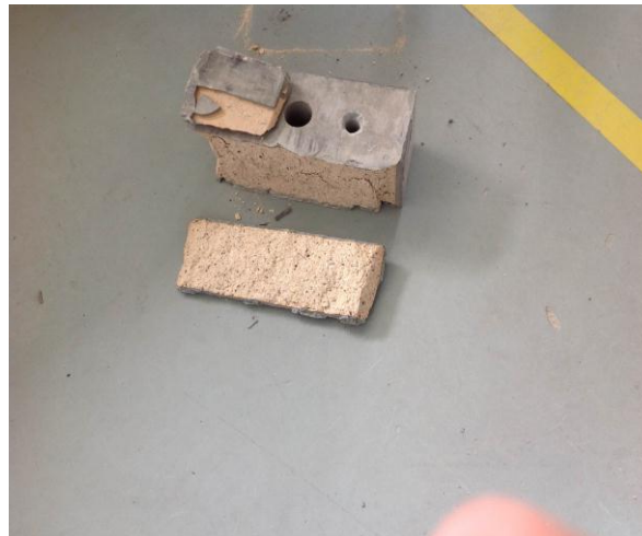
Figure 4.1 Shape of the failed brick after Compressive Strength Test
