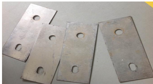
Figure 3.5 Steel plates used as a cover.
