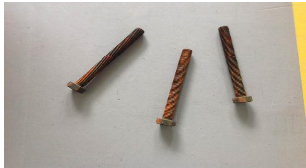
Figure 3.4 Steel rod for fastening bottom and upper brick layers.
