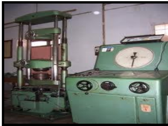
Figure 4.1 Universal Testing Machine used for testing the steel rod
