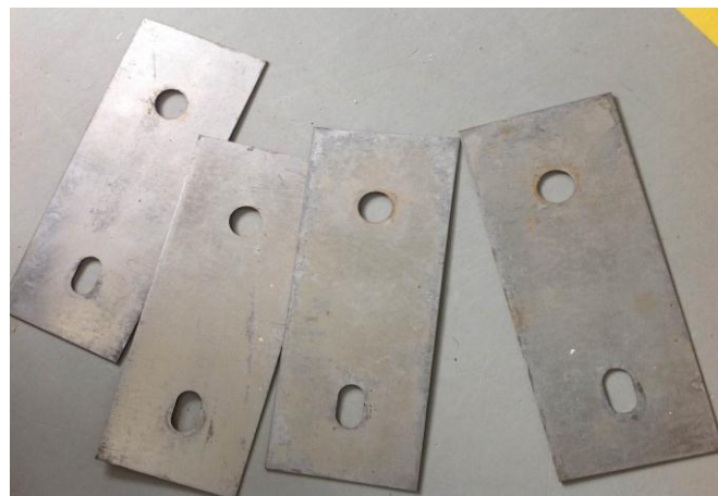
Figure 3.5 Steel plates used as a cover.
