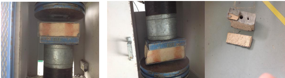
Figure 3.9 Shows the compressive strength test conducted on brick samples
