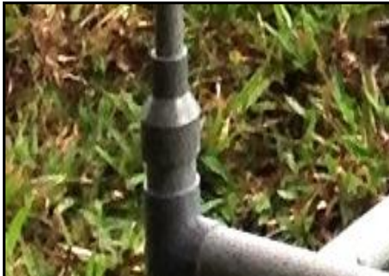
Figure 3.9: Reducers 40 mm to 20 mm diameter
