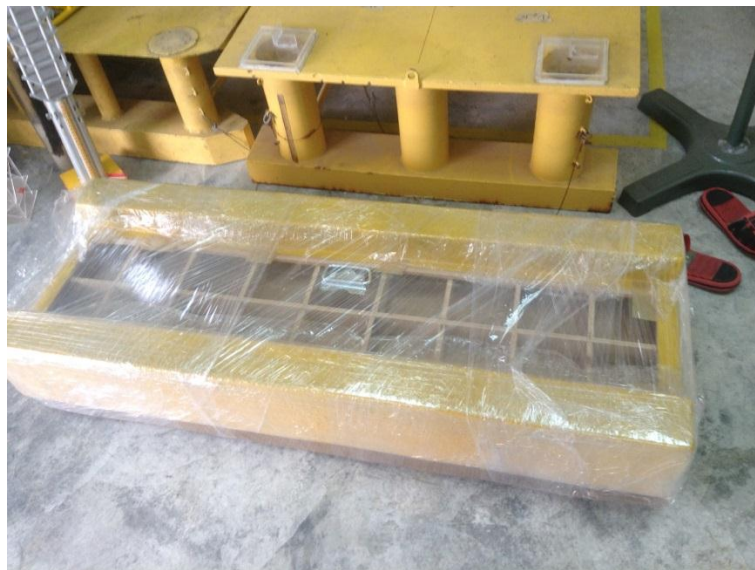
Figure 3.3 Wooden grid chambers for the placement of sandbags into floating breakwater
