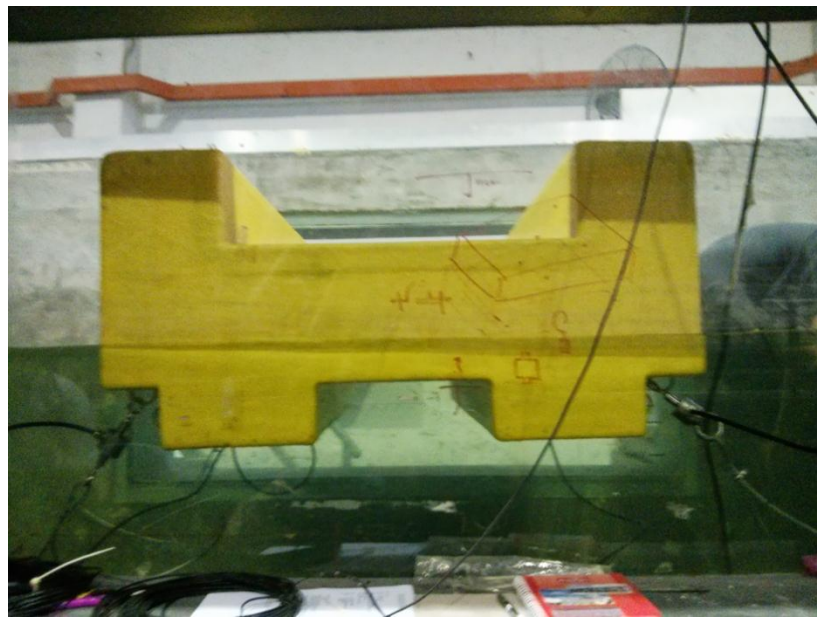
Figure 3.7: Mooring connection set up
