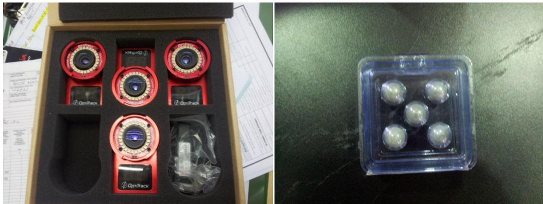
Figure 3.11: (a) Optical Tracking System camera, (b) reflective balls
