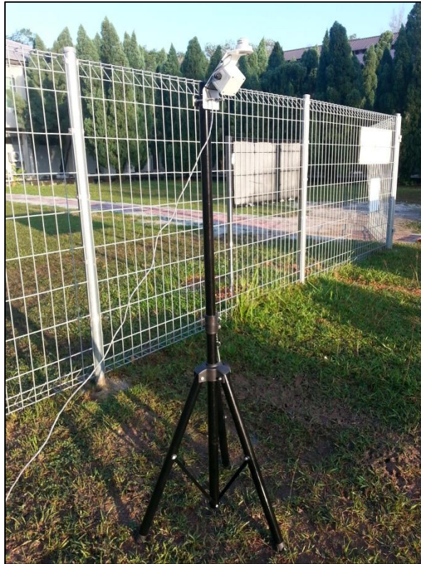
Figure 21: Solar Radiation Sensor
