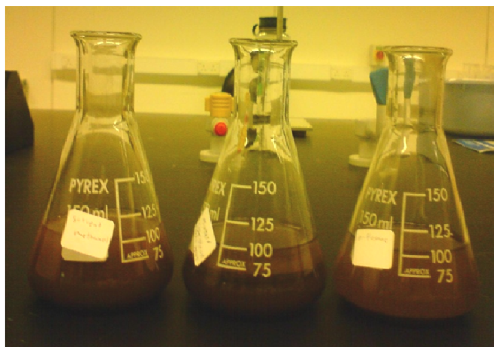
Figure 26: Settling of the mixtures of microalgae and solvents
