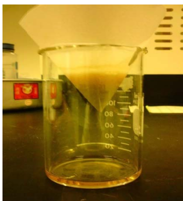
Figure 30: Separation of esterified product from sediments
