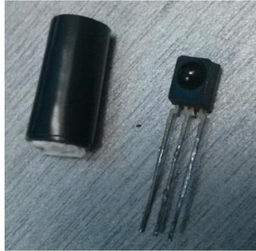
**Appendix 2: Infrared Receiver with non-reflective sleeve**
