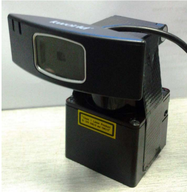
Figure 10 - The camera mounted to the laser range finder
