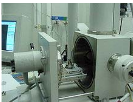
Figure18: SEM opened sample chamber. [12]
