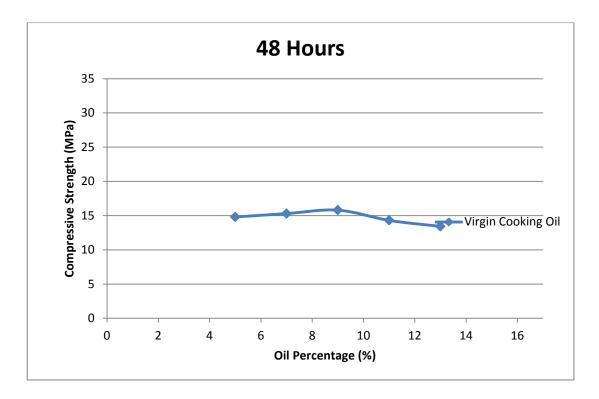
Figure 4.2 Compressive Strength of Virgin Cooking Oil Brick with 48 Hours of Curing
