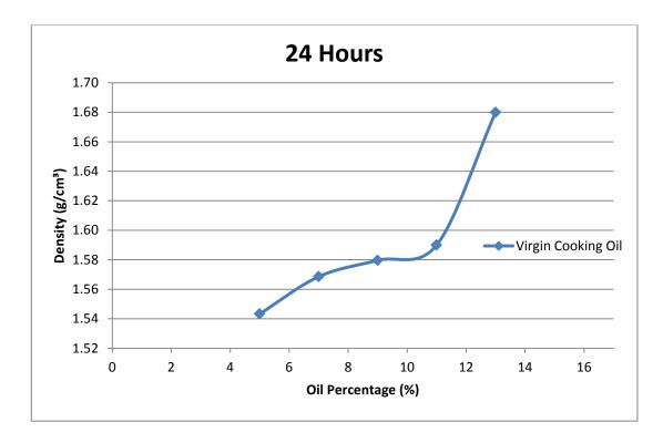
Figure 4.9 Density of Virgin Cooking Oil Brick with 24 Hours of Curing
