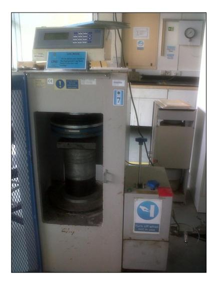
Figure 3.3 Compressive Strength Machine
