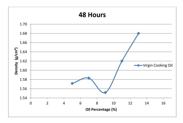
Figure 4.10 Density of Virgin Cooking Oil Brick with 48 Hours of Curing
