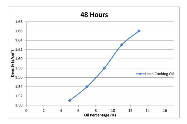
Figure 4.14 Density of Used Cooking Oil Brick with 48 Hours of Curing
