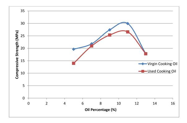
Figure 4.19 Strength of Virgin Cooking Oil Bricks and Used Cooking Oil Bricks at 72 Hours of Curing
