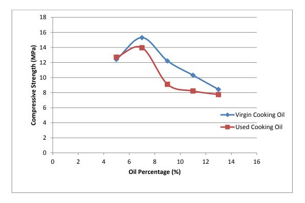
Figure 4.17 Strength of Virgin Cooking Oil Bricks and Used Cooking Oil Bricks at 24 Hours of Curing
