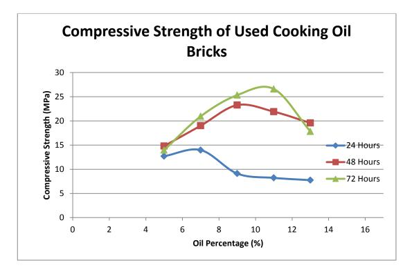
Figure 4.8 Compressive Strength of Used Cooking Oil Brick with 24, 48 and 72 Hours of Curing
