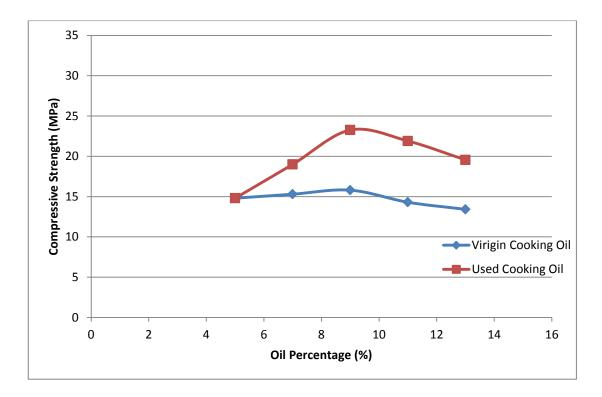
Figure 4.18 Strength of Virgin Cooking Oil Bricks and Used Cooking Oil Bricks at 48 Hours of Curing
