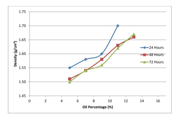
Figure 4.16 Density of Used Cooking Oil Brick with 24, 48 and 72 Hours of Curing
