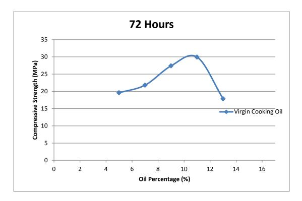
Figure 4.3 Compressive Strength of Virgin Cooking Oil Brick with 72 Hours of Curing
