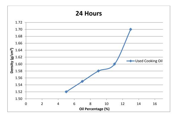
Figure 4.13 Density of Used Cooking Oil Brick with 24 Hours of Curing
