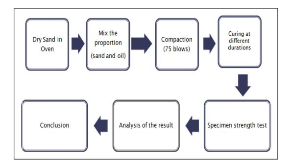
Figure 3.1 The Experimentation Process of Making Bricks Made from Used Vegetable Cooking Oil
