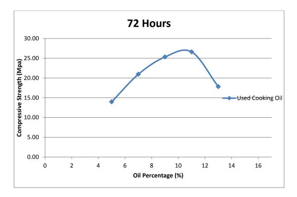
Figure 4.7 Compressive Strength of Used Cooking Oil Brick with 72 Hours of Curing
