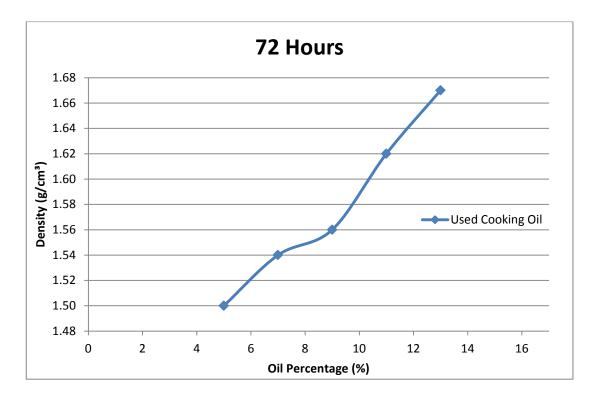
Figure 4.15 Density of Used Cooking Oil Brick with 72 Hours of Curing
