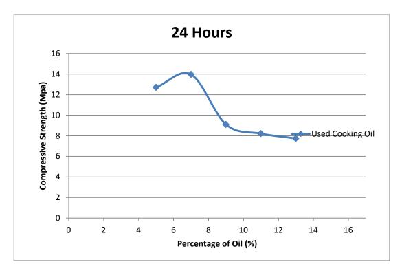
Figure 4.5 Compressive Strength of Used Cooking Oil Brick with 24 Hours of Curing
