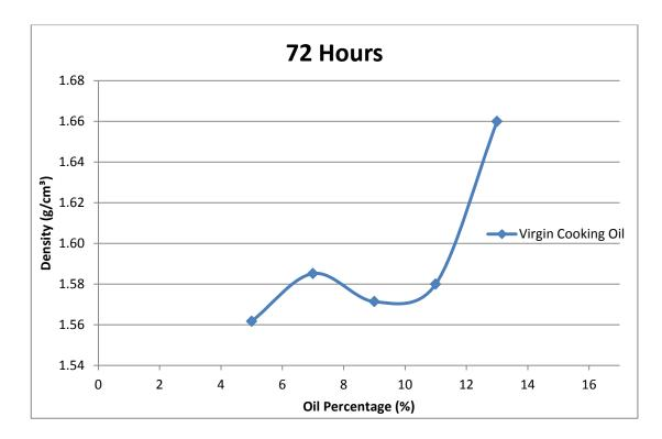
Figure 4.11 Density of Virgin Cooking Oil Brick with 72 Hours of Curing
