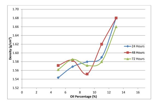
Figure 4.12 Density of Virgin Cooking Oil Brick with 24, 48 and 72 Hours of Curing
