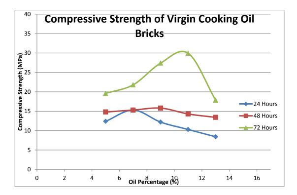
Figure 4.4 Compressive Strength of Virgin Cooking Oil Brick with 24, 48 and 72 Hours of Curing
