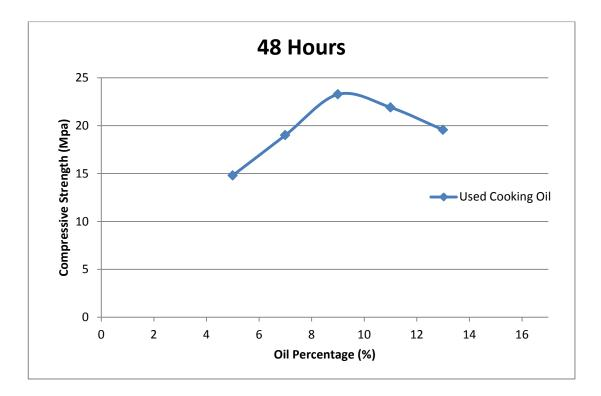
Figure 4.6 Compressive Strength of Used Cooking Oil Brick with 48 Hours of Curing
