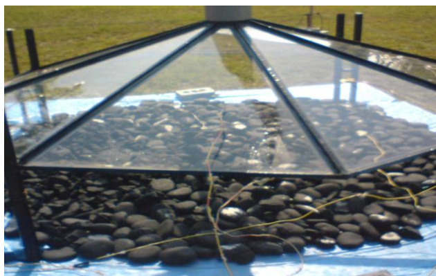
Figure 6.12: Thermocouple wires on Perspex surface for data logging
