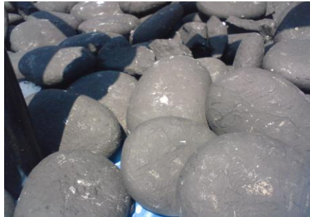
Figure 6.4: Black painted rocks as the heat collector medium of the model
