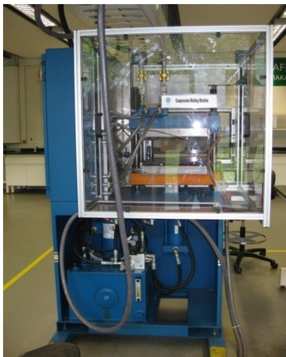
Figure 3.5: Carver Compression Molding Machine
