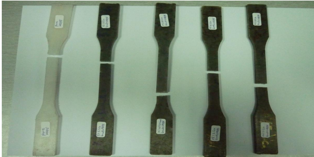
Figure 4.2: Broken Tensile Specimen of HDPE+SiO 2 composites
