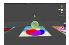
Figure 61 : mesh collider attached to the ball model
