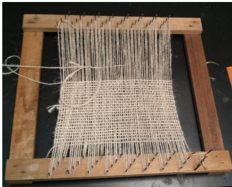
Figure 3.1.1: Woven kenaf on weaving tool.
