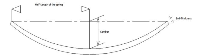
Figure 5: Specifications of Leaf Spring's Design
