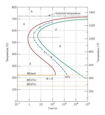
**Figure 7: Continues Cooling Transformation Diagram**
