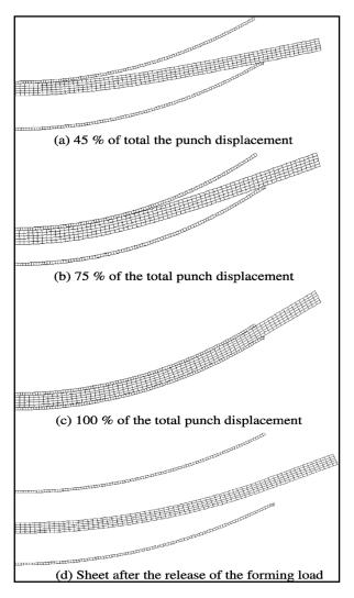
Figure 9: The Geometry of the Sheet Metal by Percent of Forming Load
