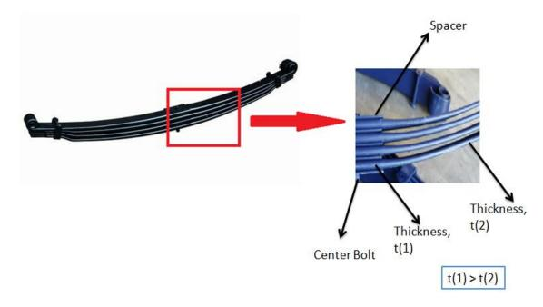
**Figure 2: Sample of Parabolic Spring**
