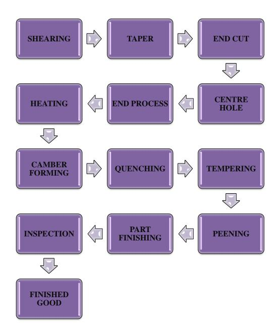
Figure 3: Process Flow of Leaf Spring Manufacturing
