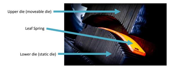
Figure 4: A view of Finger-Press Camber Forming Machine
