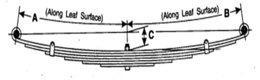
Figure 1: Sample of Multileaf Spring (C is notation for camber)
