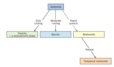
**Figure 8: Flow of producing Tempered Martensite**
