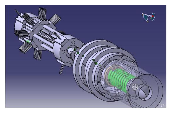
Figure 23: Complete model of PIG drive mechanism after correction.
