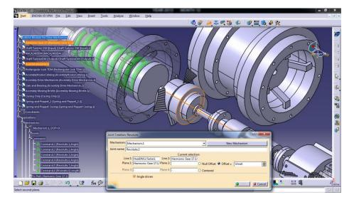
Figure 33: Revolve joint for Harmonic gear and HUD.
