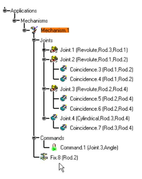
Figure 16: The fixed part is identified in the specification tree. [10]
