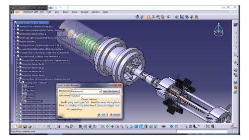
Figure 42: Prismatic joint for moving bristle and poppet casing.
