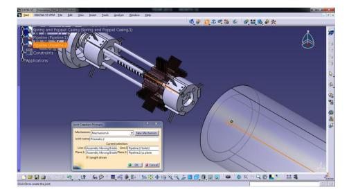
Figure 50: Example Prismatic joint for mechanism 4 (Moving Bristle with Pipeline).
