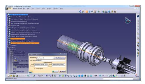
Figure 46: Prismatic joint for Poppet and Turbine casing.
