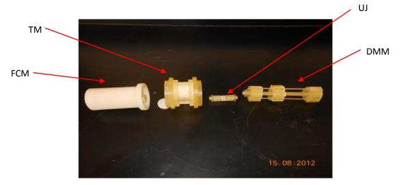
Figure 1: Photo shot of PIG prototype design assembly arrangement. [4]
