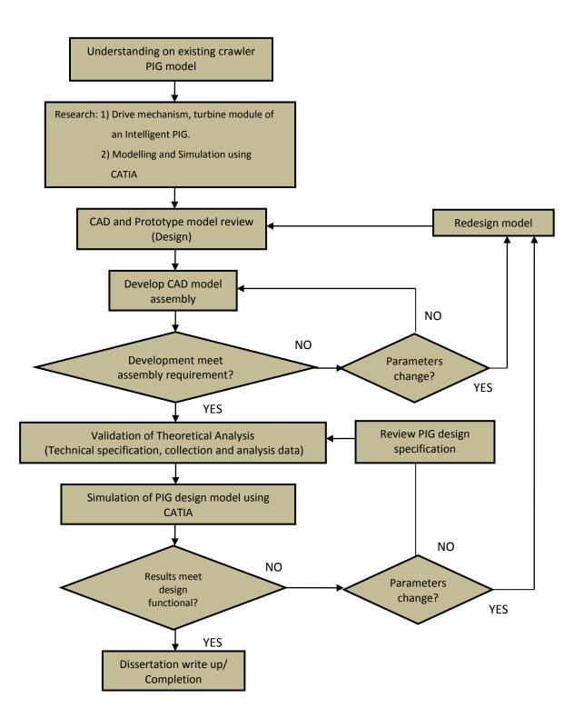
Figure 20: Flowchart of PIG Simulation
