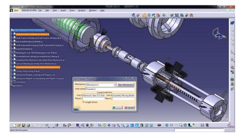
Figure 37: Prismatic joint for Harmonic gear and moving bristle.
