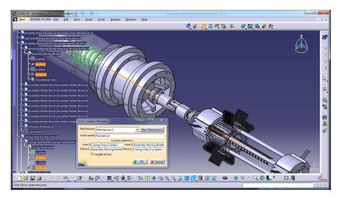
Figure 41: Prismatic joint for moving bristle and turbine casing.
