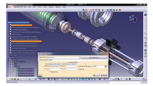
Figure 35: Revolve joint for Harmonic gear and Cam.
