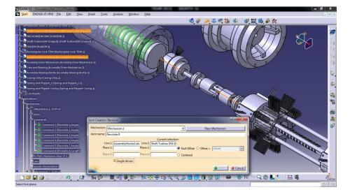
Figure 36: Revolve joint for Harmonic gear and Shaft.
