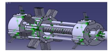
Figure 22: Drive Mechanism module with aligned holder bar. [7]
