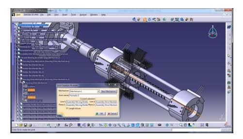
Figure 43: Prismatic joint for moving bristle and holder bar with brush holder.
