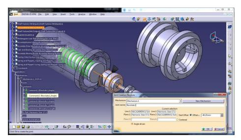
Figure 32: Revolve joint for Harmonic gear and Turbine blade.
