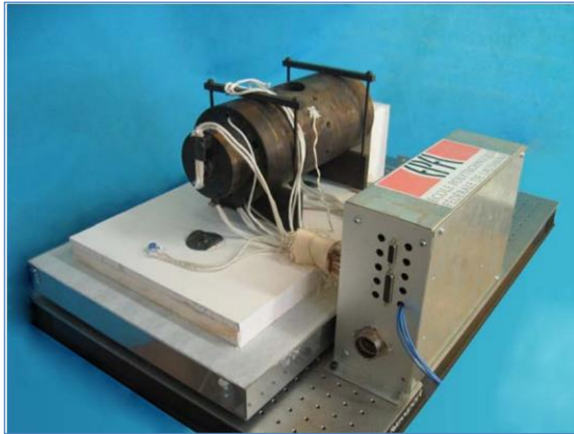
Figure 2.6: Equipment to test magnetic bearing at high temperature
