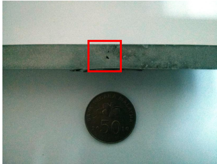
Figure 4. 2: Worm tunnel defect in Pass A.
