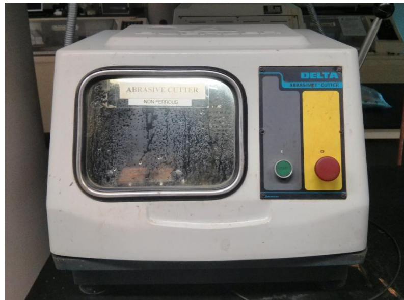
Figure 3. 14: Abrasive cutter is used to section small workpiece.
