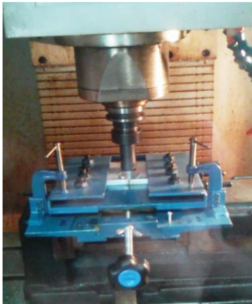
Figure 3. 10: The workpiece is been weld by the welding tool.
