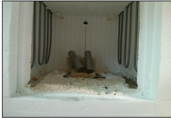
Figure 3. 3: Tool steel H13 is placed inside the furnace with heating element on both sides
