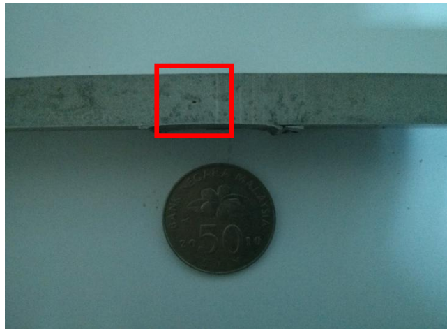
Figure 4. 4: Presence of worm hole defects in Pass B
