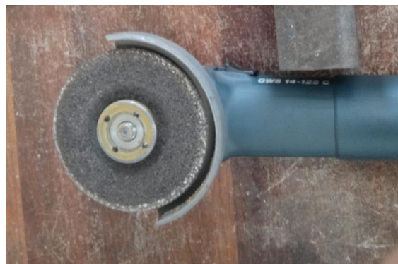
Figure 3. 12: Hand grinder is used to remove flash.
