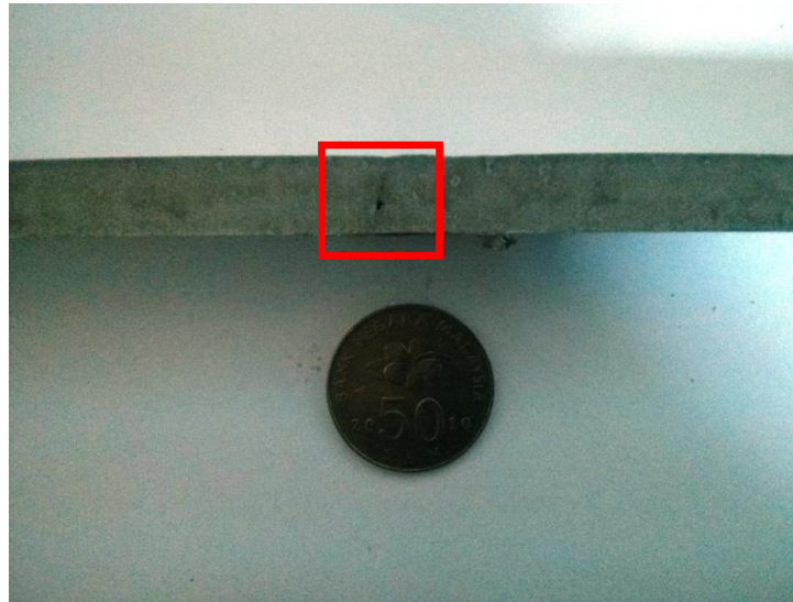
Figure 4. 6: Worm tunnel in Pass C welded plate.
