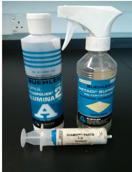
Figure 3. 19: Diamond particle used during polishing process
