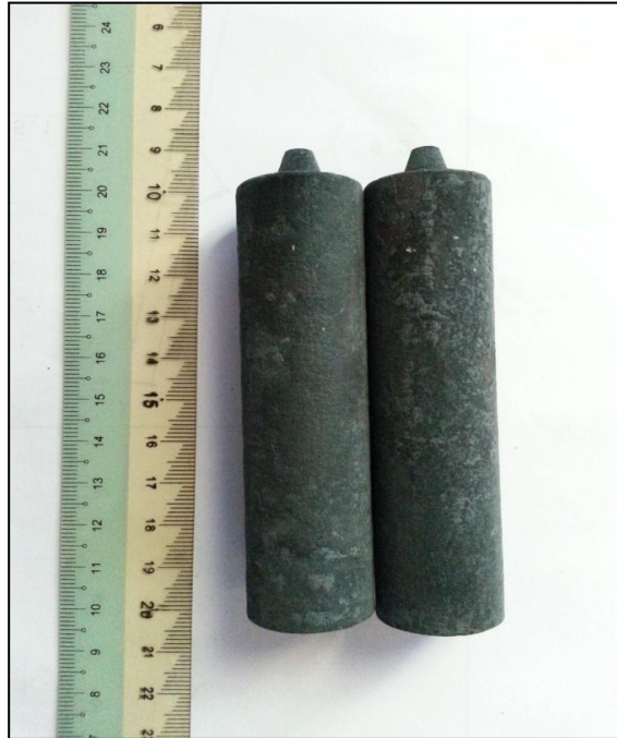
Figure 3. 5: Condition of tool steel H13 after preheat, austenitize and air quench
