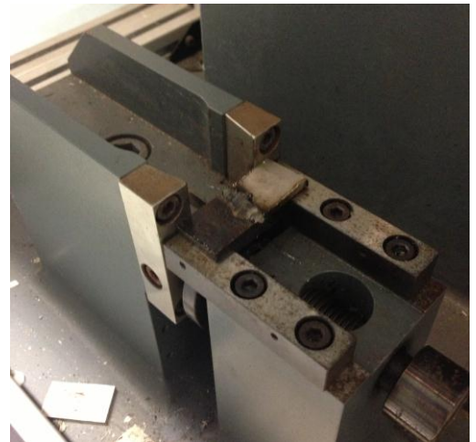
Figure 27: Placement of the sample on the anvil
