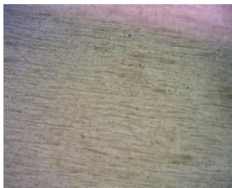
Figure 31: Microstructure at Stainless steel HAZ
