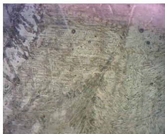
Figure 32: Microstructure at Weld Zone
