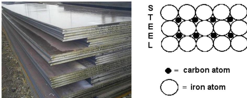
Figure 10: Steel Plate and atomic structure of carbon steel (Lansky,2013)
