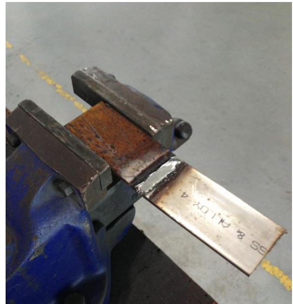
Figure 18: Sample was clamped for grinding
