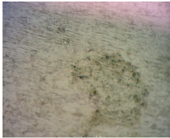
Figure 28: Microstructure at Stainless steel HAZ
