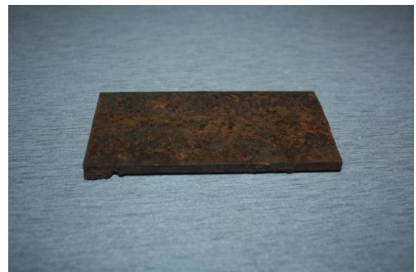
Figure 14: Mild Steel Plate (100x50mm)
