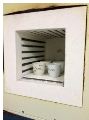
Figure 8 : Catalyst was calcined in the furnace at 800C
