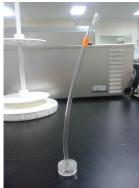
FIGURE 4 SPECIMEN AFTER MOUNTED IN EPOXY
