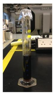
Figure 3.8 : Samples of Water-in-Oil Emulsion
