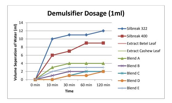
Figure 4.10 : Performance Plot for 1 ml Dosage for Different Type of Demulsifier
