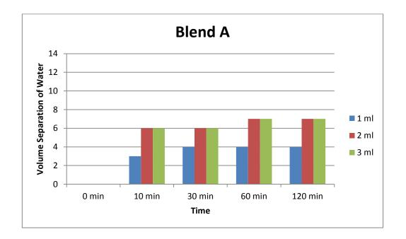
Figure 4.5 : Volume Separation of Water using Blend A
