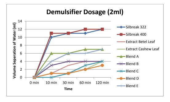
Figure 4.11 : Performance Plot for 2 ml Dosage for Different Type of Demulsifier
