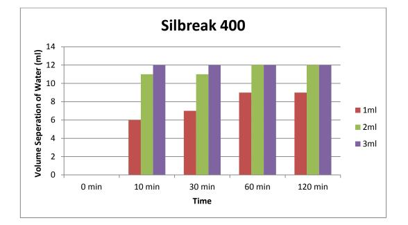
Figure 4.2 : Volume Separation of Water using Sillbreak 400
