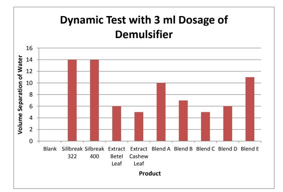
Figure 4.13 : Dynamic Test Result using 3ml Dosage of Demulsifier
