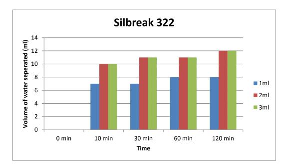
Figure 4.1 : Volume Separation of Water using Sillbreak 322
