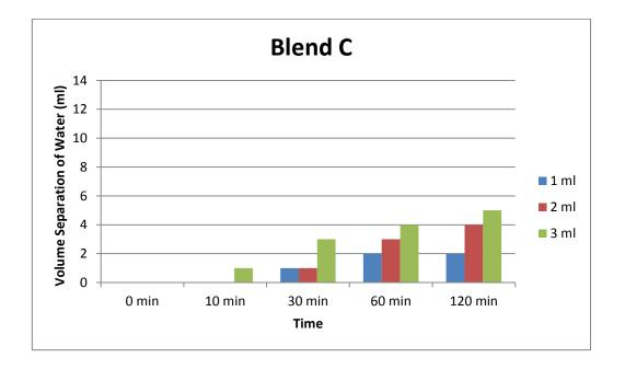
Figure 4.7 : Volume Separation of Water using Blend C
