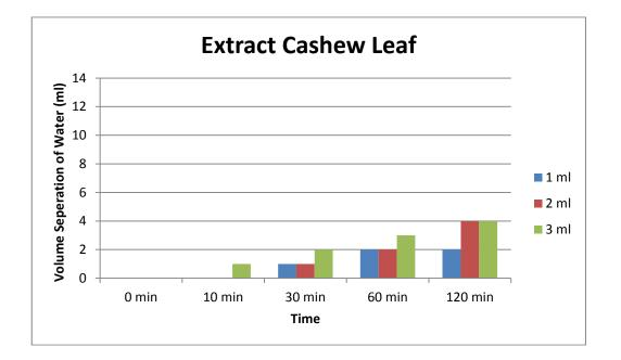
Figure 4.4 : Volume Separation of Water using Extract Cashew Leaf
