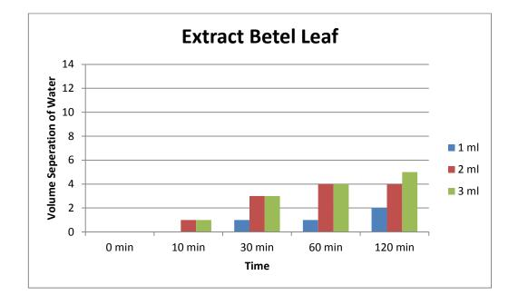
Figure 4.3 : Volume Separation of Water using Extract Betel Leaf
