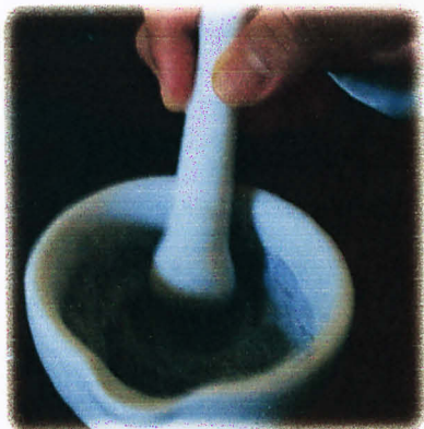
Figure 11: The dried catalyst is comminuted in order to enhance the effectiveness of the calcination process
