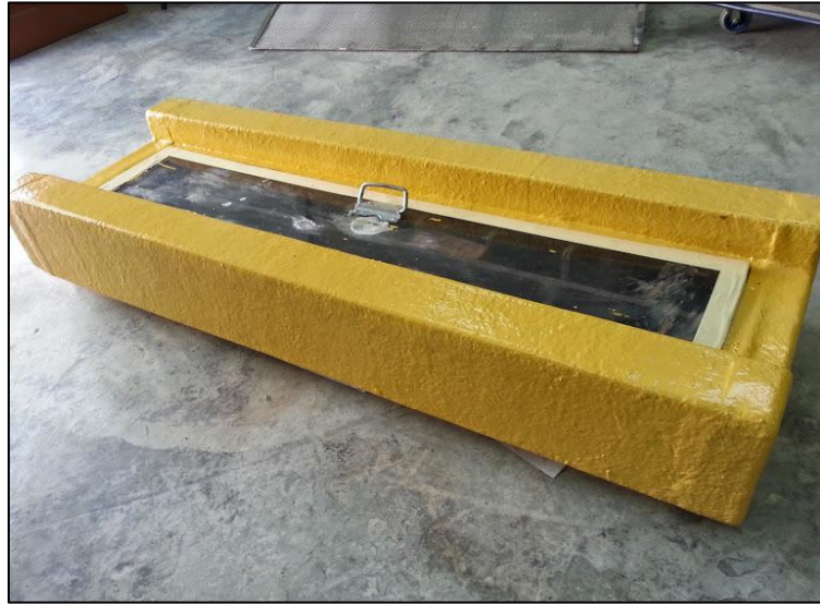
Figure 3.4: Fabricated H-float model
