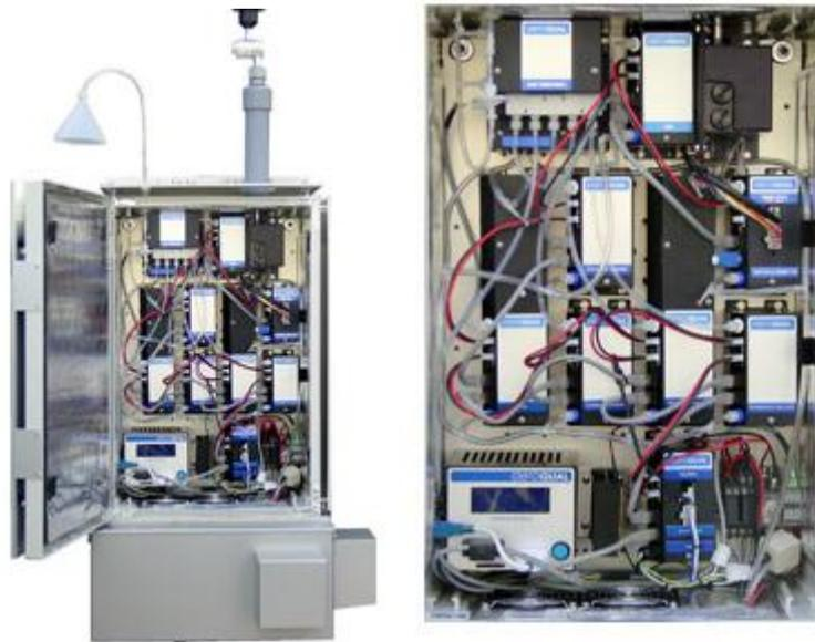
Figure 5: Aeroqual AQM60 Environmental Station
